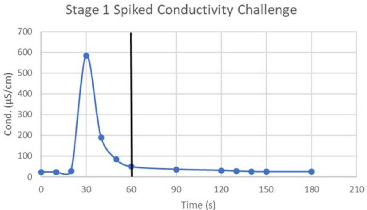
Figure 4-6. Stage 1 “Time-of-Flight” Study to Determine Solenoid Sample Duration.
