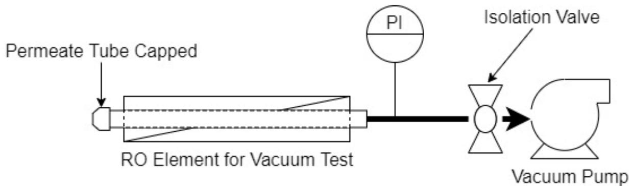
Figure 8-4. Schematic of a Vacuum Decay Test for an RO or NF Membrane Element.
