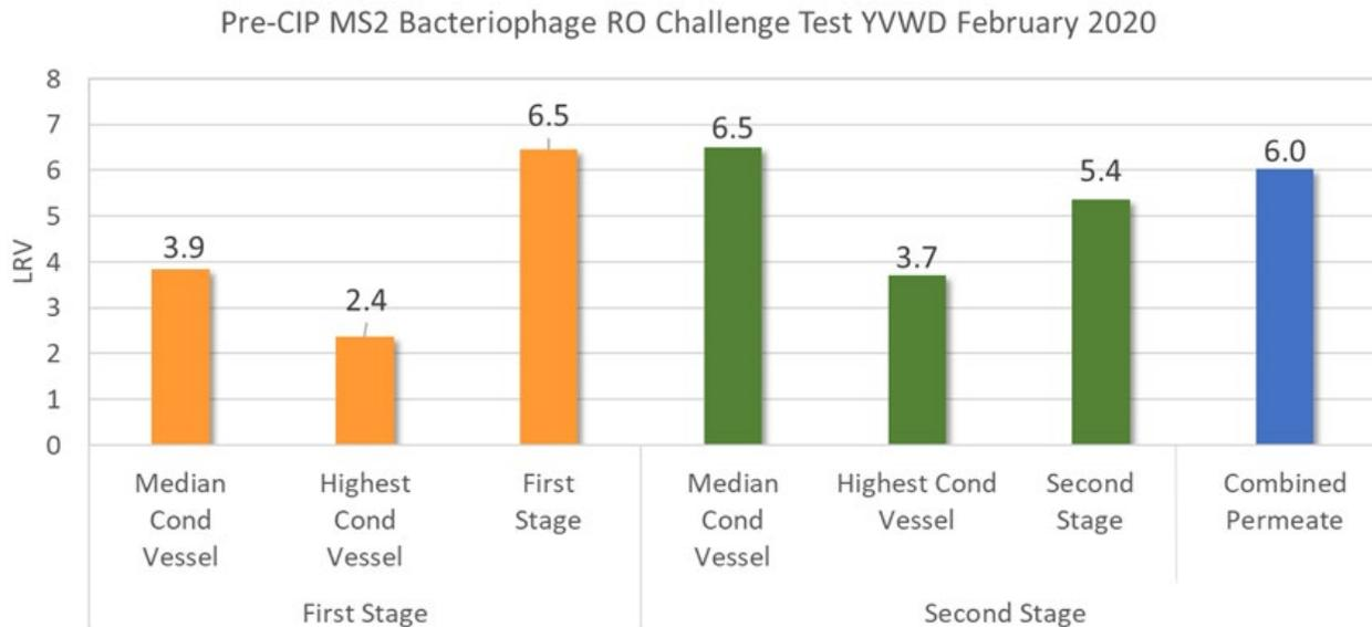
**Figure 6-11. MS2 LRVs Attained by the YVWD RO System During Test 1 - Pre-CIP MS2 Test.**
