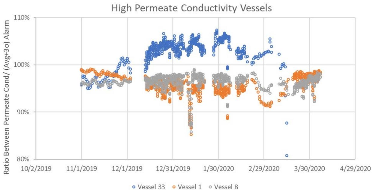
**Figure 4-9. Ratio of the Vessel Permeate Conductivity to the Average + 3 $\sigma$  Alarm.**
