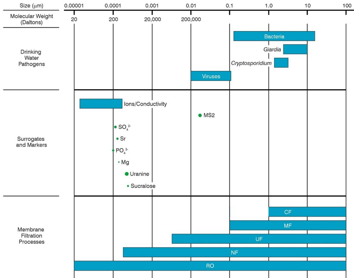
Figure 1-1. Modified Filtration Application Guide for Pathogen Removal Indicating Size of Surrogates Evaluated in This Study.
