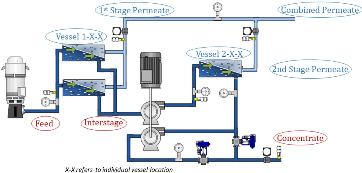
Figure 6-3. Sampling Locations of the YVWD RO System.
