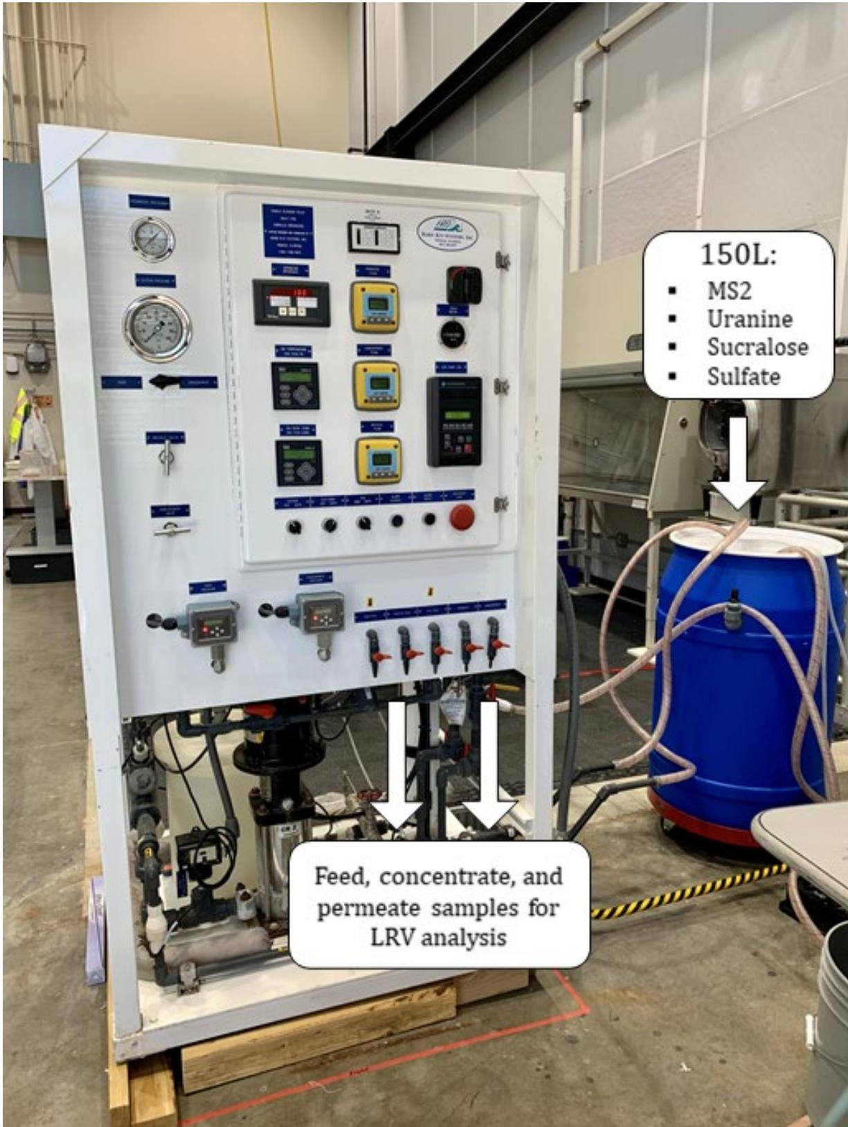
Figure 8-1. The Single-Element Pilot Skid and 150L Synthetic Feed Reservoir Used During Challenge Testing Experiments at SNWA.
