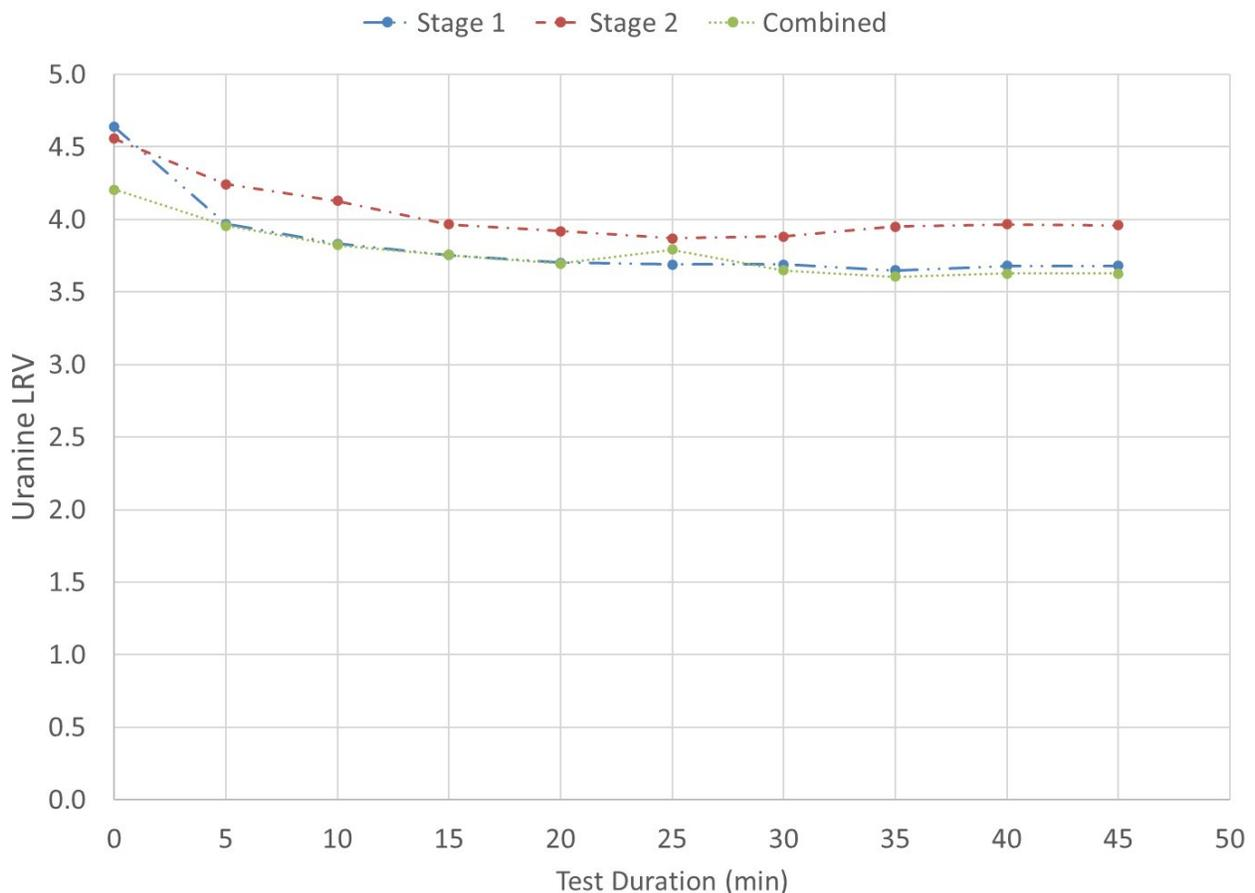
**Figure 7-9. Uranine LRVs During Challenge Testing of the WCWA Pilot RO.**
