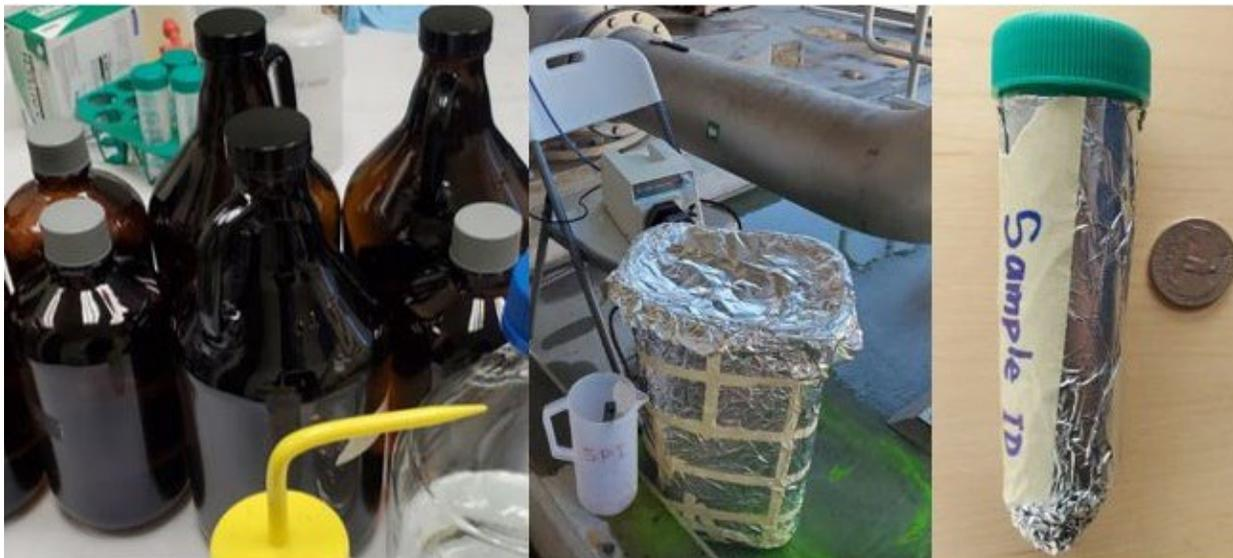
**Figure 6-9. Dilutions, Uranine Stock Solution, and Sample Tubes.**
