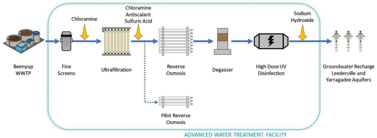
**Figure 7-1. Beenyup Groundwater Replenishment Process Flow Diagram.**
