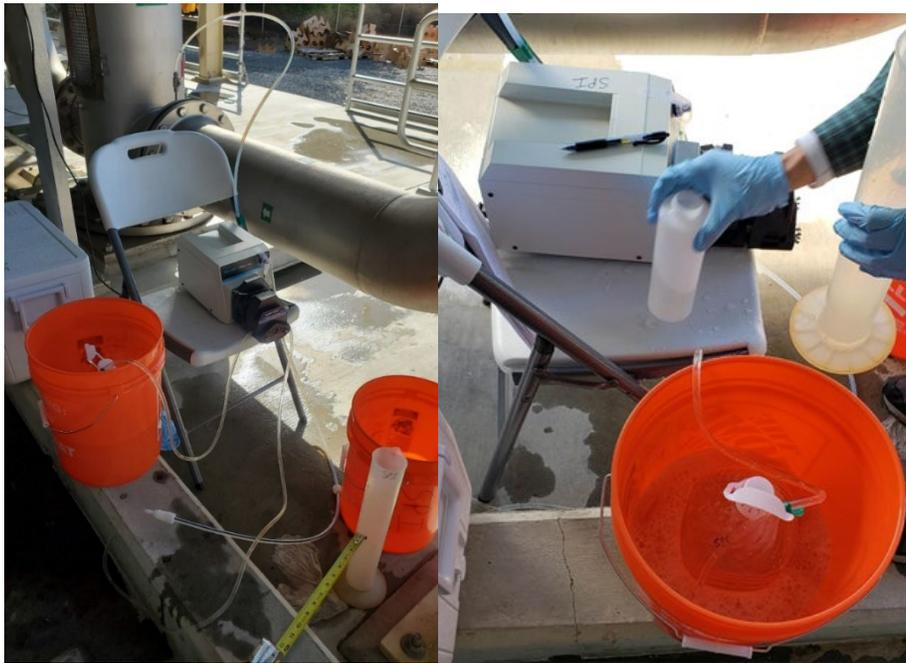
Figure 6-5. MS2 Pumping Setup Upstream of RO High-Pressure Feed Pump at YVWD.
