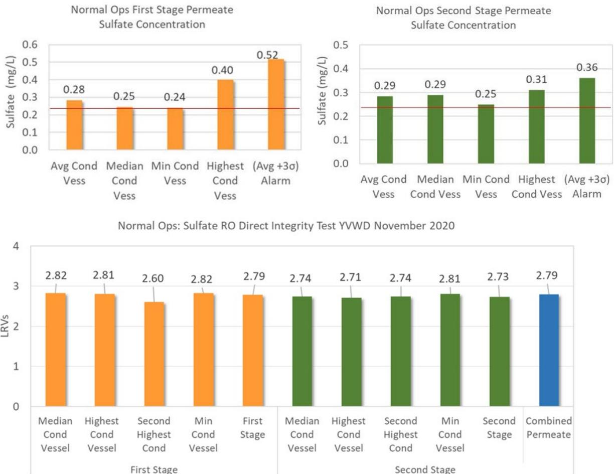
**Figure 6-23. Sulfate LRVs Attained by the YVWD RO During Normal Operation - Test 7.**
