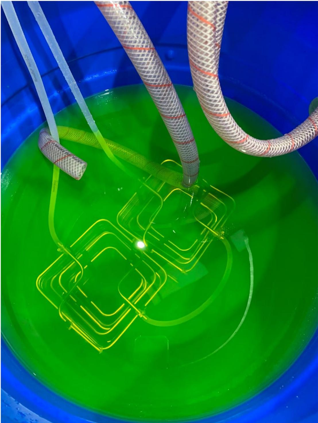
Figure 8-6. Photo of the Feed Bucket Containing the Uranine Dosed for the Tail Test Condition.
