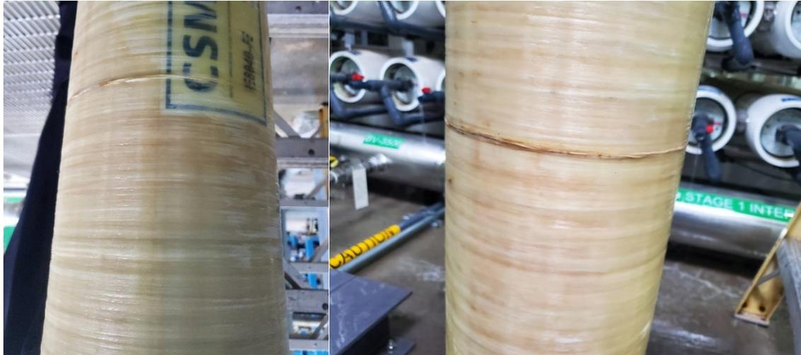
**Figure 4-11. Cracked Tail element of Vessel 33.**
