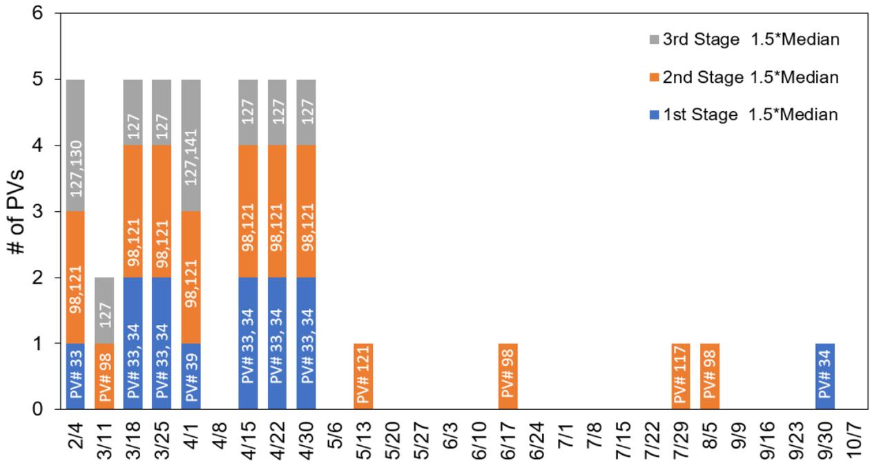
**Figure 5-4. Number of RO Pressure Vessels Observed with Permeate EC 1.5\*Median per RO Stage for each Conductivity Profiling Event.**
