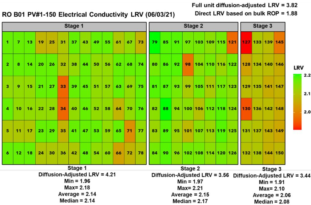
Figure 5-15. Color Heat Map of the LRVs Calculated from Individual PV Permeate EC Concentrations. Sampling Completed on 6/3/2021.
