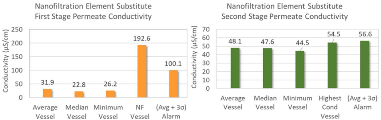
**Figure 6-16. Manual Conductivity Profile Prior to MS2 Dosing for Test 4 - NF Element Substitution.**
