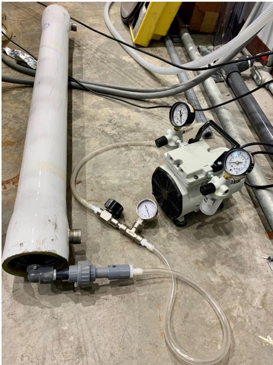
Figure 8-5. Picture of the Vacuum Hold Test Performed at SNWA.
