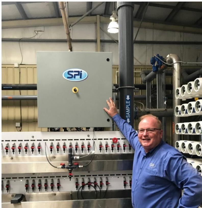
Figure 4-5. Automated Conductivity Profiling Apparatus at YVWD.
