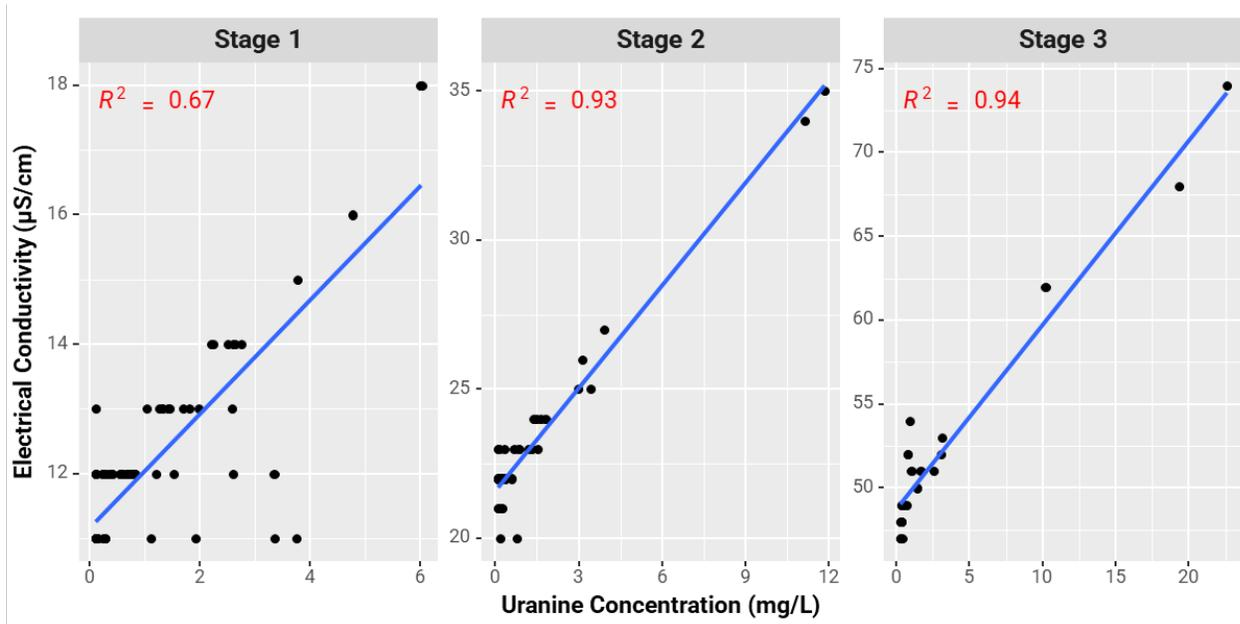
Figure 5-16. Correlation of EC Versus Urinine for each Individual Pressure Vessel's Permeate Sampled on 06/03/21.
