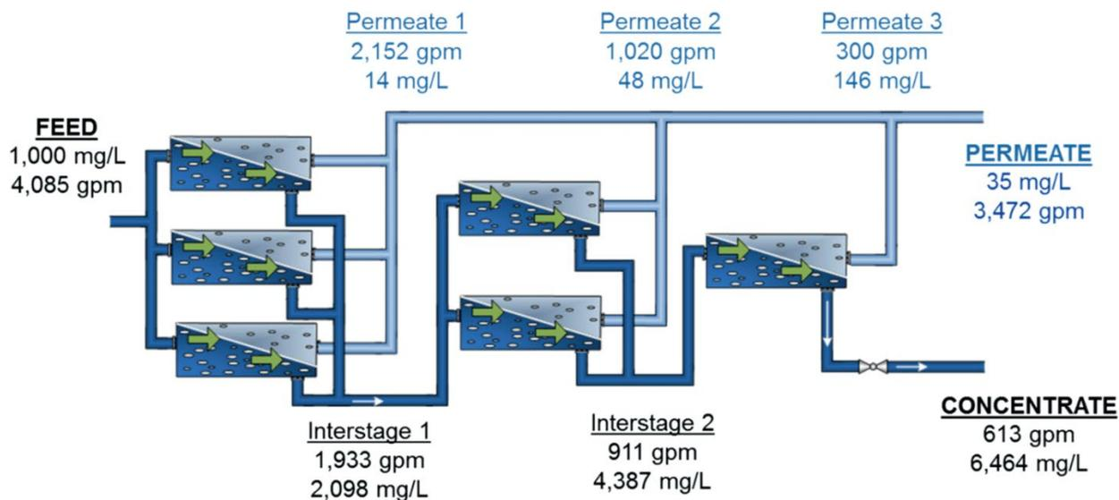
Figure 5-1. Typical Three-Stage Reverse Osmosis Unit and Instrumentation at the OCWD GWRS AWWP.
