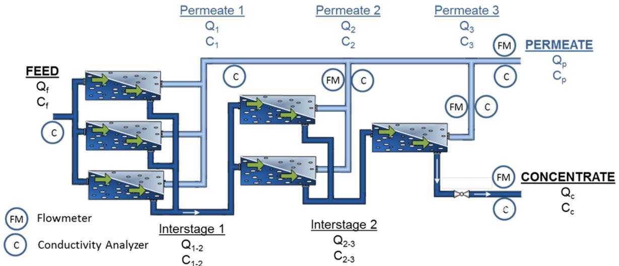
Figure 2-1. Typical Three-Stage Reverse Osmosis Unit Instrumentation.
