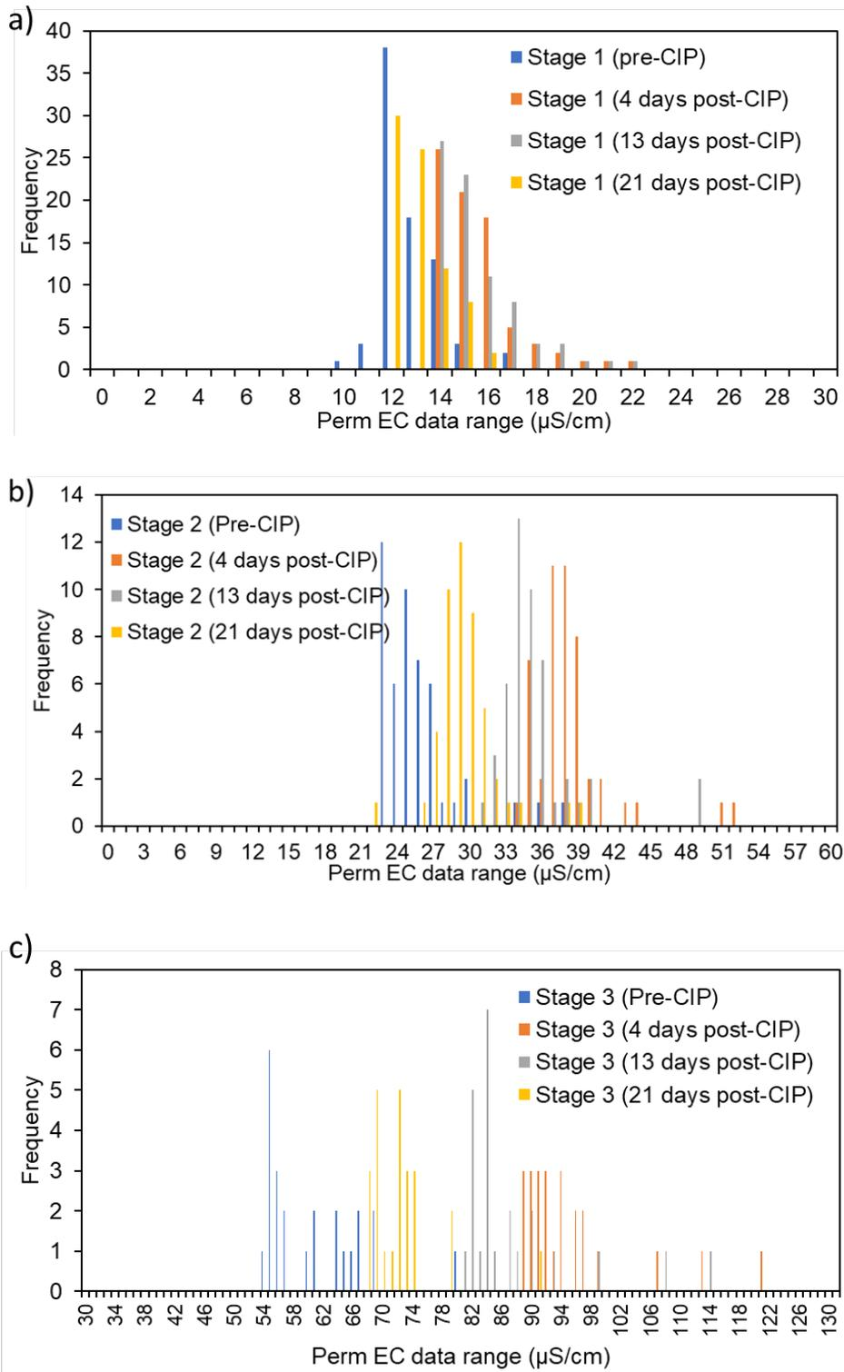
**Figure 5-7. Impact of CIP on EC Profiling for a) Stage 1, b) Stage 2 and c) Stage 3 for the Array Studied at OCWD.** (Sampling completed on 5/13, 2021 [pre-CIP] and 5/16/2021 and 5/21/2021 [post-CIP]). Tick marks (bin) on x-axis indicate the permeate EC and the y-axis (“frequency”) indicates the number of pressure vessels that produce permeate with the corresponding EC.
