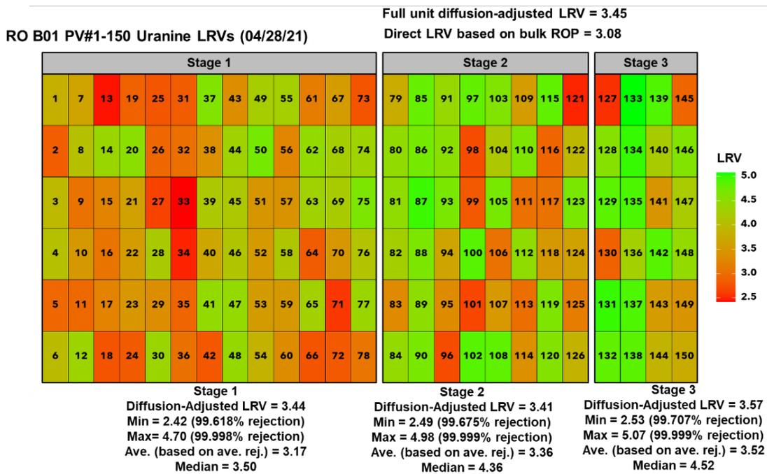
**Figure 5-11. Color Heat Map of the LRVs Calculated from the Individual PV Permeate Uranine Concentrations. Sampling Completed on 4/28/2021.**
