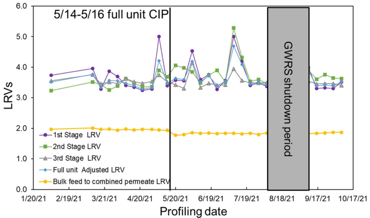
**Figure 5-5. OCWD EC Profiling Calculated LRV for the 1st Stage, 2nd Stage, 3rd Stage, and Overall (Full Unit).**
