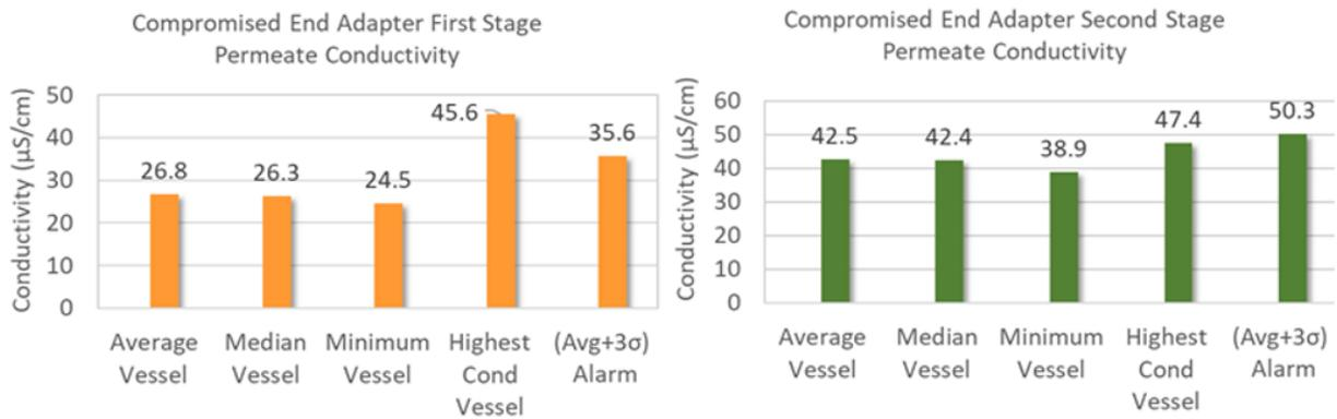
**Figure 6-12. Manual Conductivity Profile Before MS2 Dosing for Test 2 - Compromised End Adapter.**
