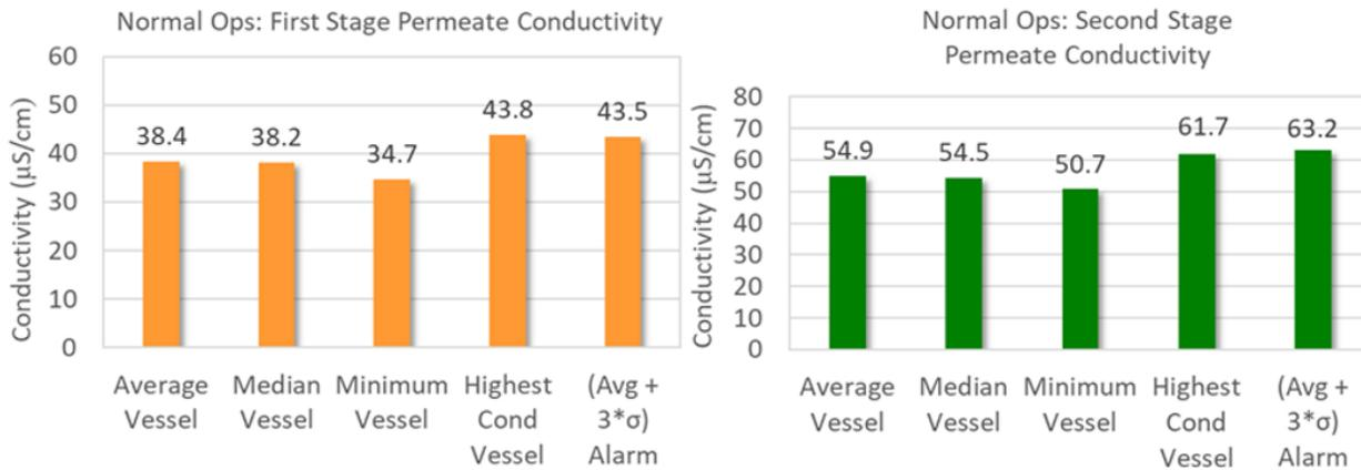
**Figure 6-18. Conductivity Profile of the YVWD RO Prior to Normal Operation - Tests 5 (MS2), 6 (Uranine), and 7 (Sulfate).**
