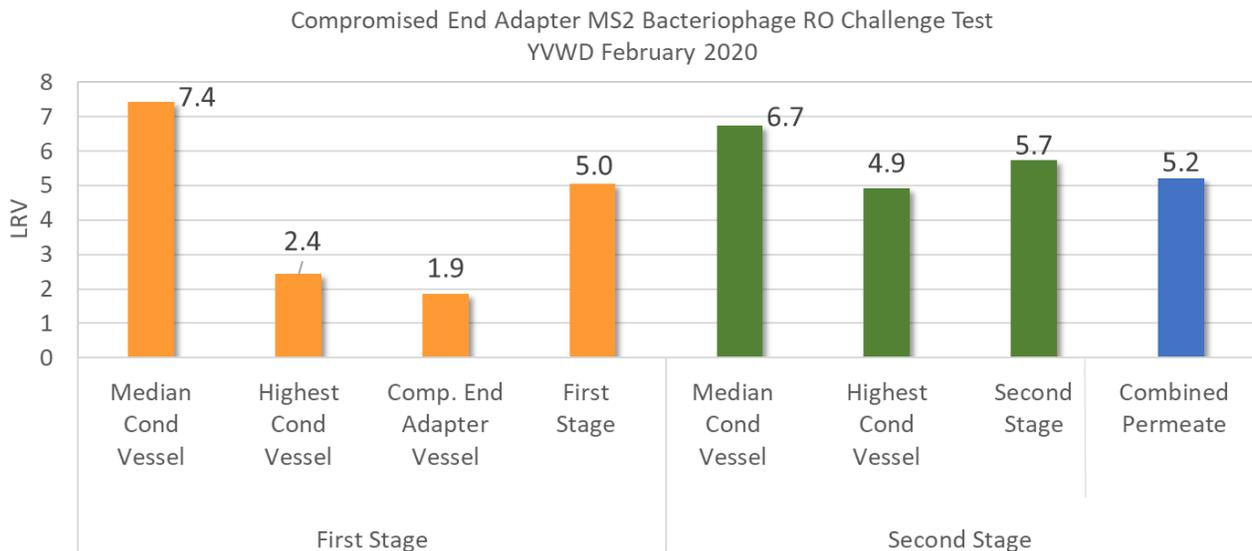
**Figure 6-13. MS2 LRVs Attained by the RO System During Test 2 - Compromised End Adapter.**
