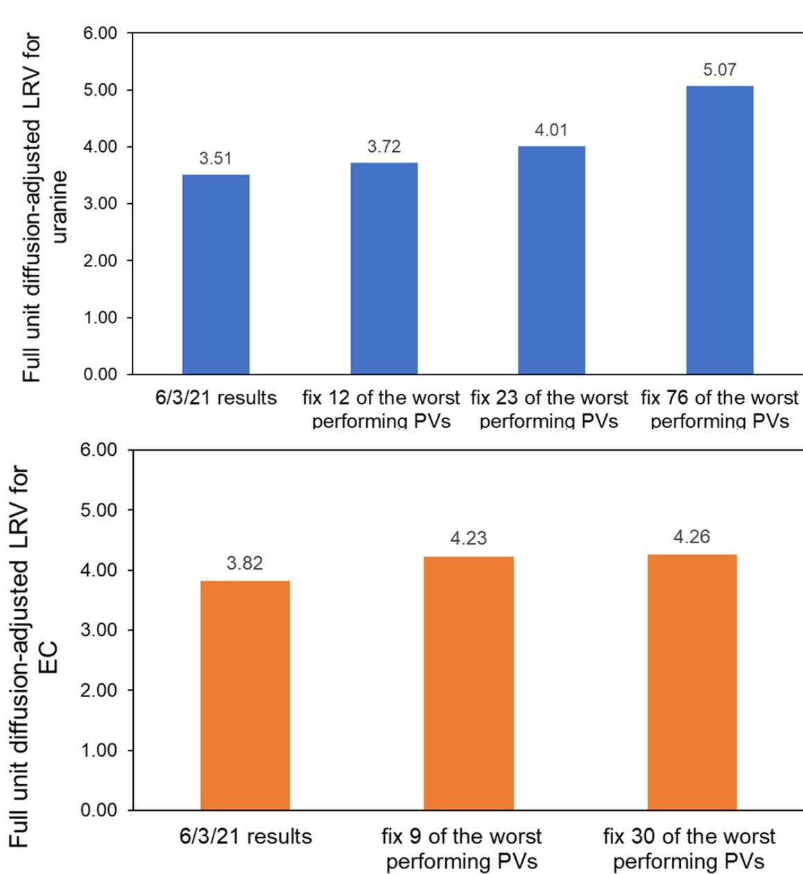
Figure 5-17. The Observed (6/3/21) and Theoretical (for Two or Three Hypothetical Cases) Full Unit LRV Calculated from Profiling Results for Uranine (Top Figure) and EC (Bottom Figure).
