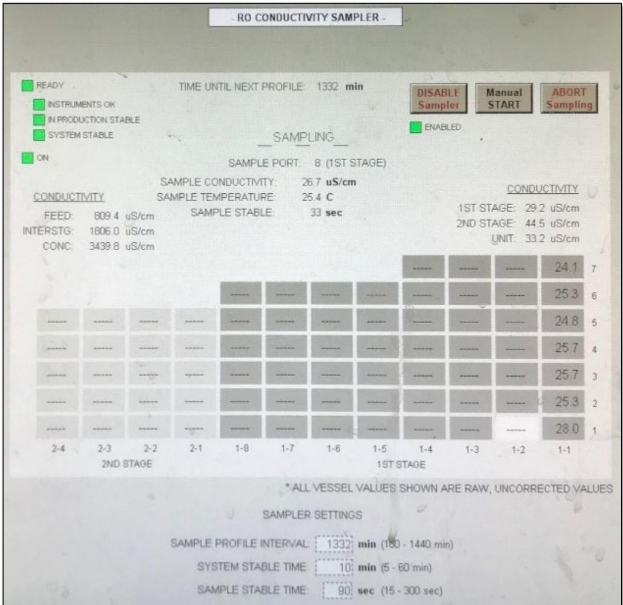
**Figure 4-7. Example of RO Automated Conductivity Profile SCADA Screen.**
