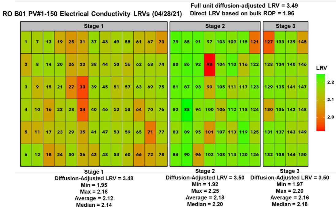
**Figure 5-12. Color Heat Map of the LRVs Calculated from the Individual PV Permeate EC Concentrations. Sampling Completed on 4/28/2021.**
