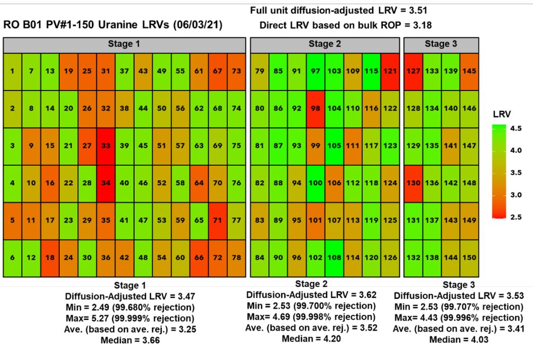
Figure 5-14. Color Heat Map of the LRVs Calculated from Individual PV Permeate Uranine Concentrations. Sampling Completed on 6/03/2021.
