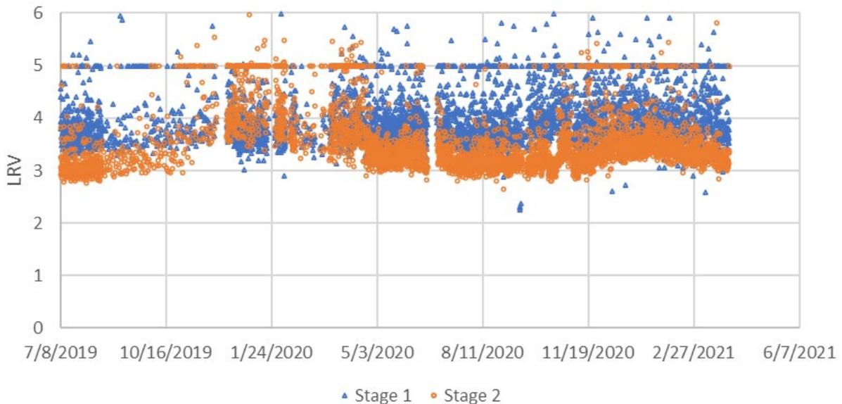
**Figure 4-16. YVWD Stage 1 and Stage 2 LRV Calculated from Conductivity Profiling Results Demonstrating more than 2.8-Log For each Stage.**
