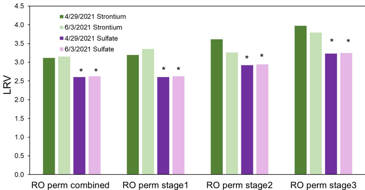
**Figure 5-18. Sulfate and Strontium LRVs for the OCWD Full-Scale RO Test Unit.**
