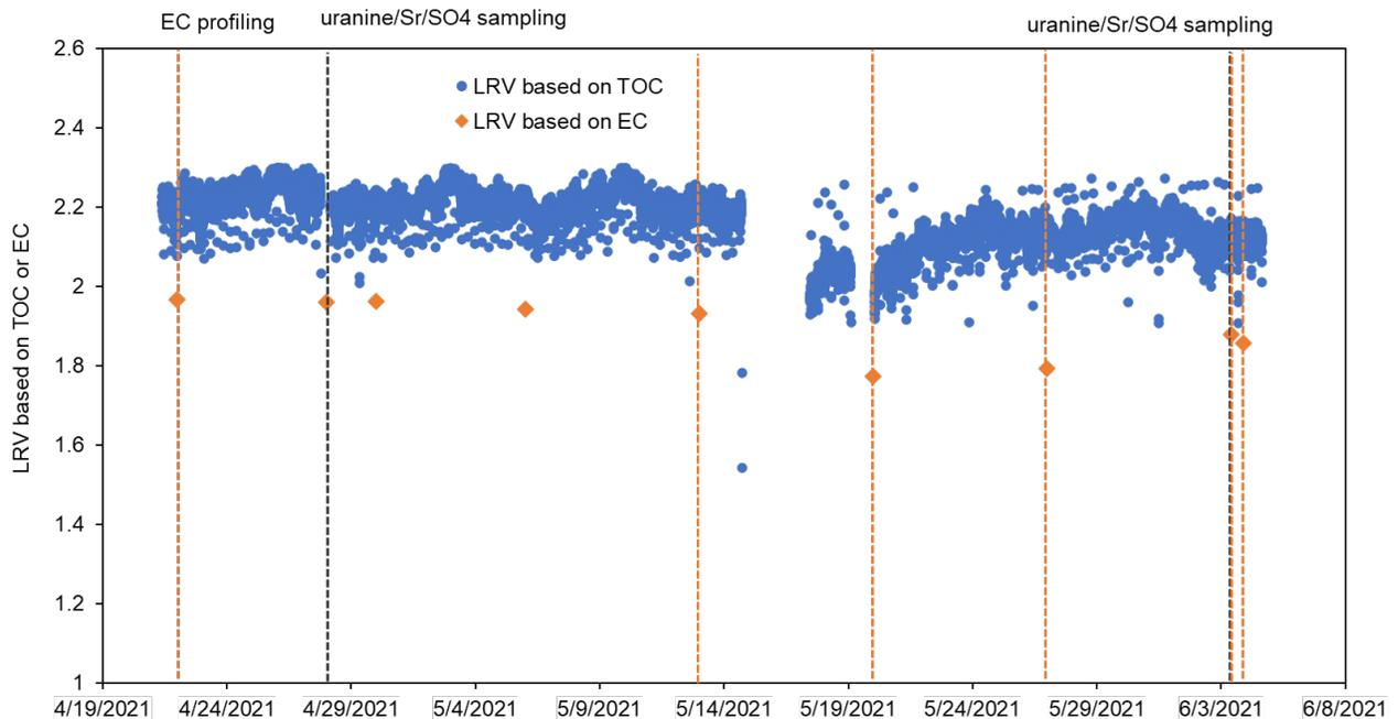
**Figure 5-8. OCWD Full-Scale Test RO Unit LRV Based on Continuous Online TOC Measurement.**
