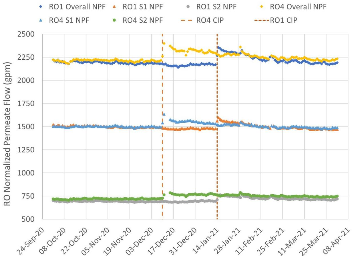
**Figure 7-2. NPF for the RO Skids Evaluated During the Trial.**
