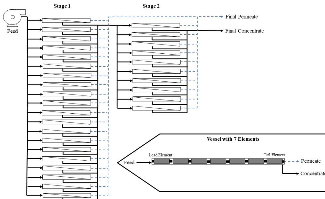
**Figure 8-3. Illustration of an Example 20:10 Array Showing the Positions of the Membrane Elements That Were Simulated in this Study.**
