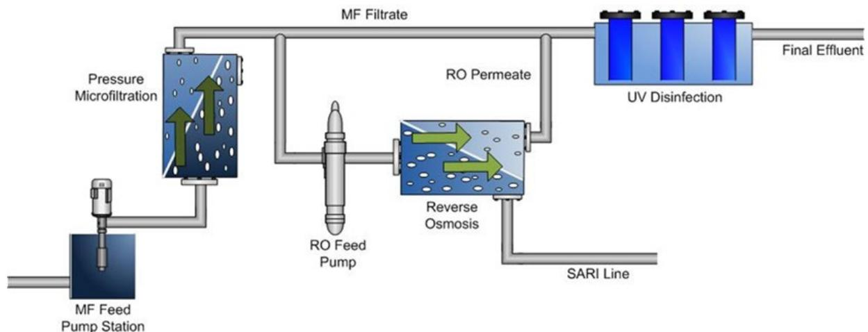
Figure 6-1. Schematic of the Wochholz Regional Water Recycling Facility.
