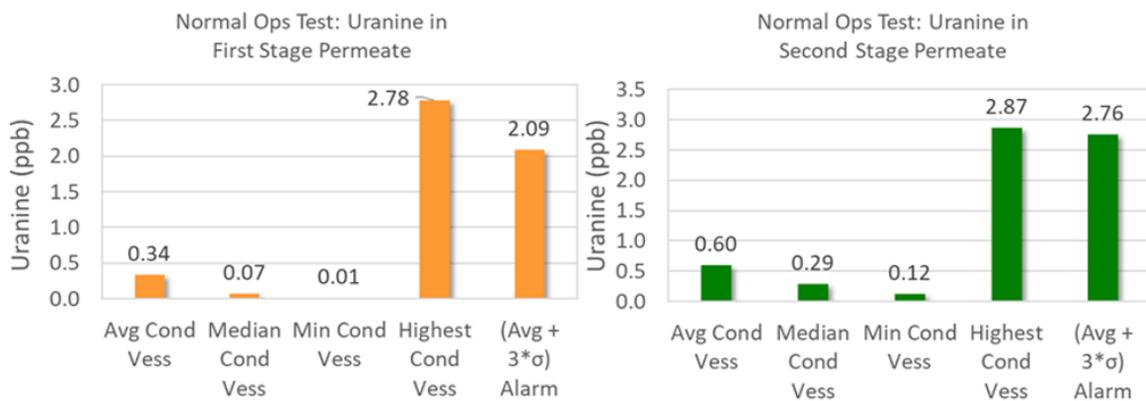
**Figure 6-21. Uranine Profile of YVWD RO System During Normal Operation - Test 6.**
