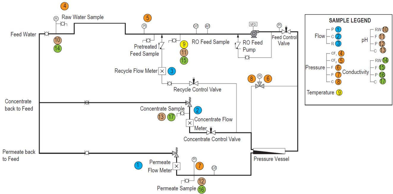
**Figure 8-2. Process Flow Diagram of the Single-Element Pilot Skid Used at SNWA.**
