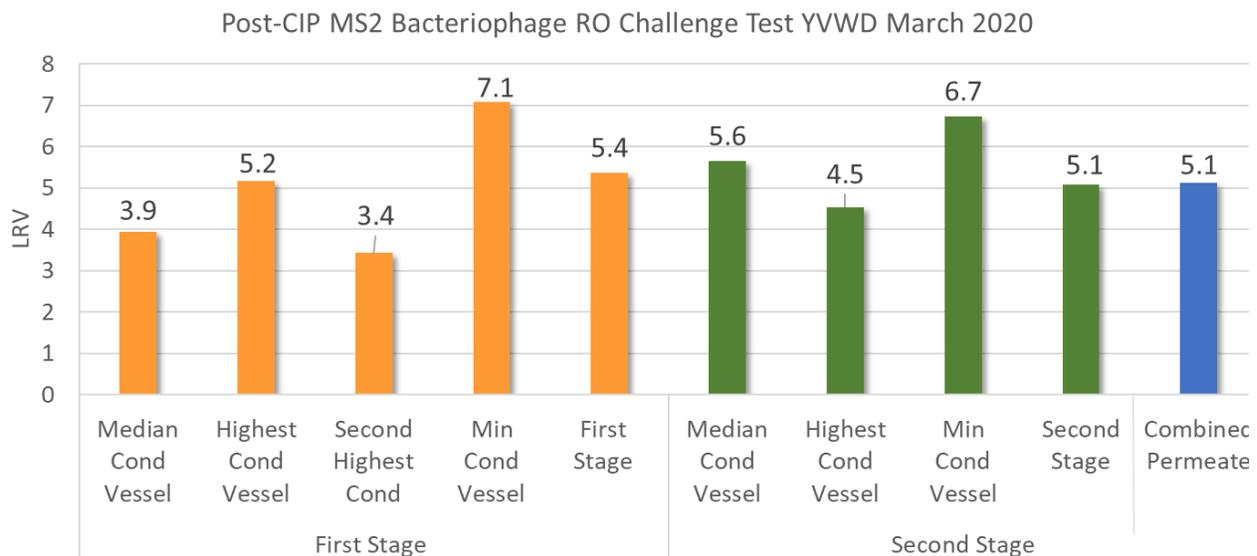
**Figure 6-15. MS2 LRVs Attained by RO System During Test 3 - Post-CIP.**
