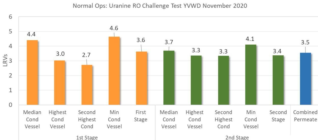
**Figure 6-22. Uranine LRVs Attained by RO System During Normal Operation - Test 6.**
