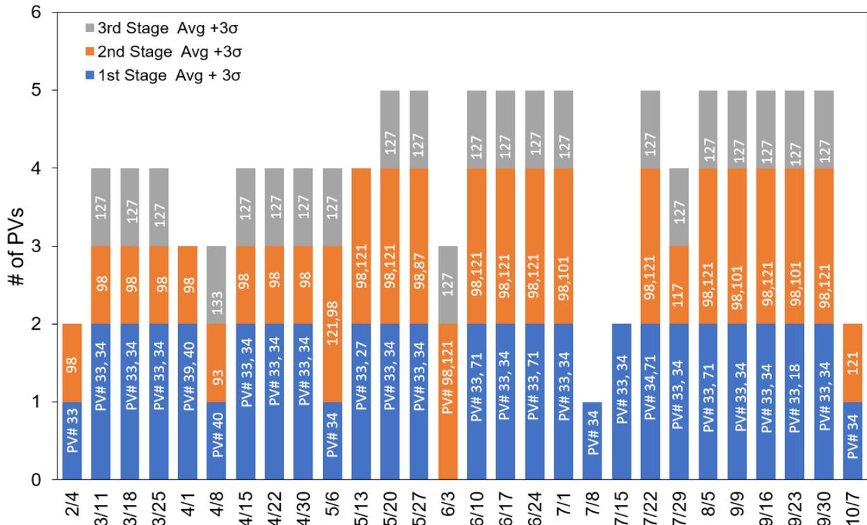
**Figure 5-3. Number of RO Pressure Vessels Observed with Permeate EC Exceeding the Limit of Average + 3σ per RO Stage for each Conductivity Profiling Event.**
