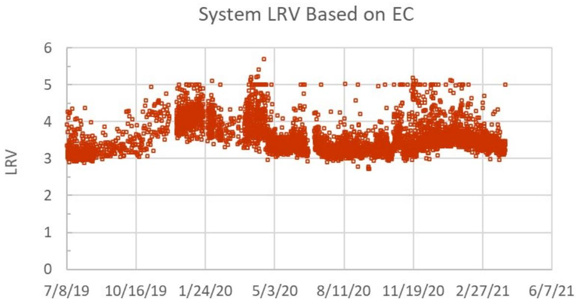
**Figure 4-17. Overall System LRV Calculated from Conductivity Profiling at YVWD Demonstrating more than 3-log.** Seasonal variation in profiling LRV is observed. Note that combined RO feed to permeate LRV was close to 1.4 indicating a sensitivity improvement by conductivity profiling of more than 1.6-log.
