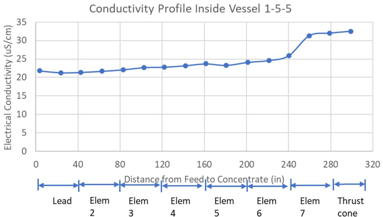
**Figure 4-10. Permeate Conductivity Measurements Inside Pressure Vessel Number 1-5-5 During Probing.**
