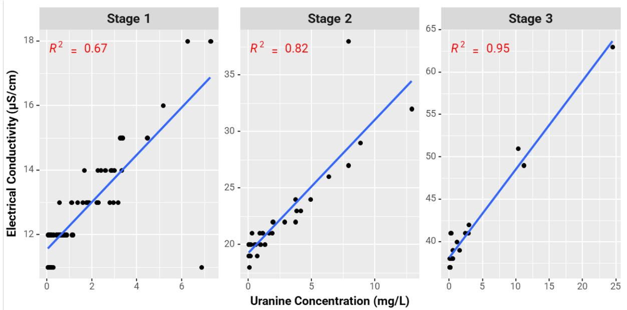
Figure 5-13. Correlation of EC Versus Uranine for each Individual Pressure Vessel's Permeate Sampled on 04/28/21.
