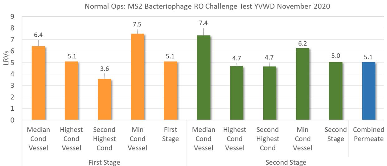
**Figure 6-19. MS2 LRVs Attained by the YVWD RO System During Normal Operation - Test 5.**
