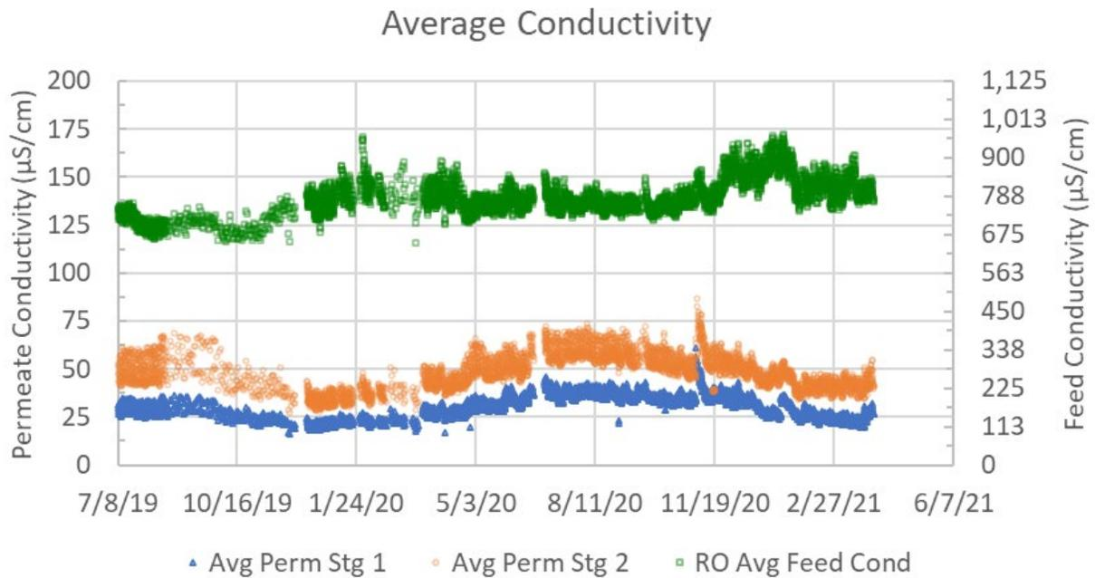
**Figure 4-13. Long Term RO Feed and Permeate Conductivity for the YVWD RO.**
