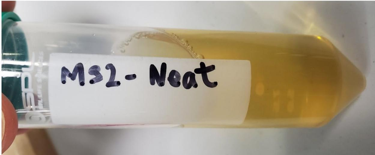
**Figure 6-4. Sample of MS2 Bacteriophage Neat Solution as Sent from GAP EnviroMicrobial Services.**
