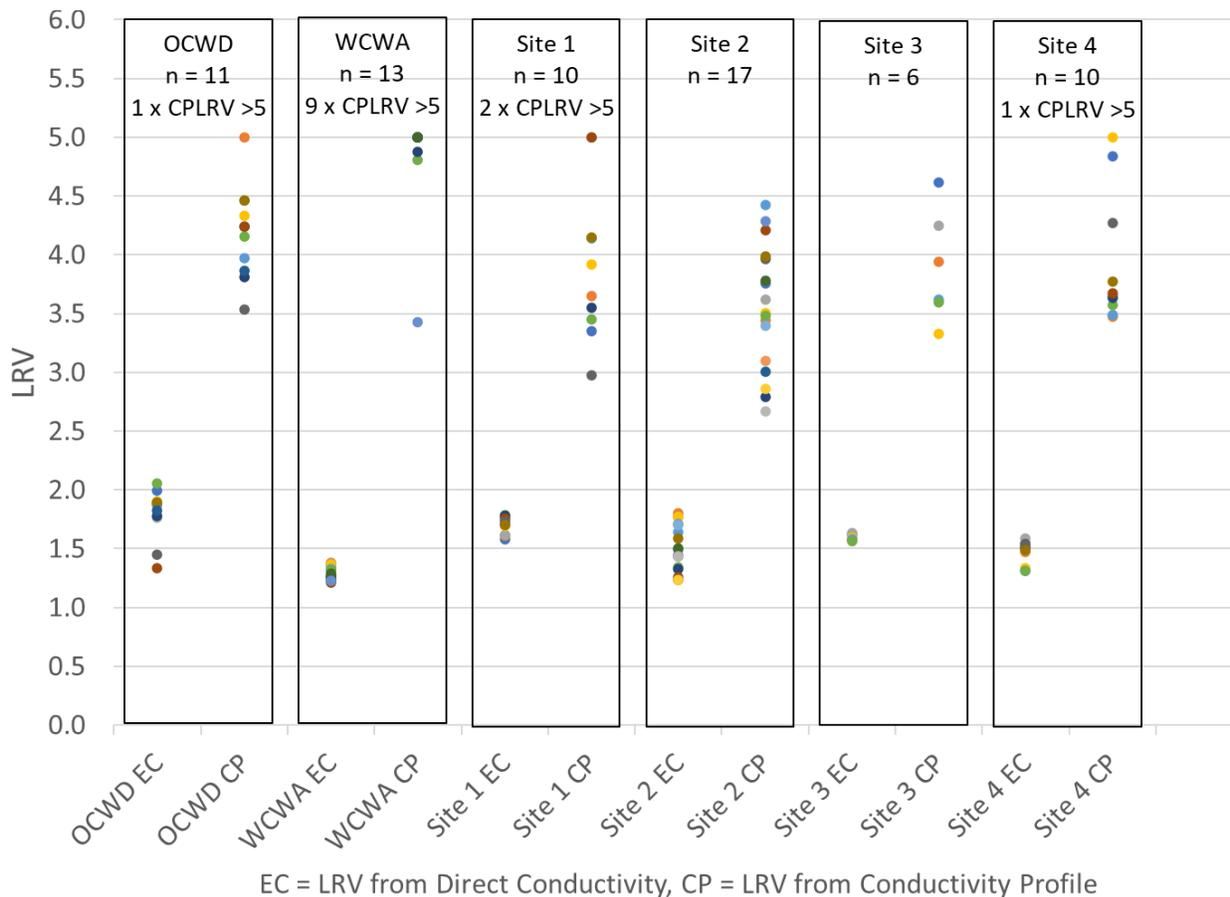
**Figure 4-18. Comparison of Conductivity Profile LRVs (CP) vs Direct Conductivity LRVs (EC) from Multiple Sites.** Typically, CP LRVs were greater than 3-log, representing a 1 - 2-log increase in LRV sensitivity compared to the direct LRV calculation method. Dots of the same color at the same site are from the same data set.
