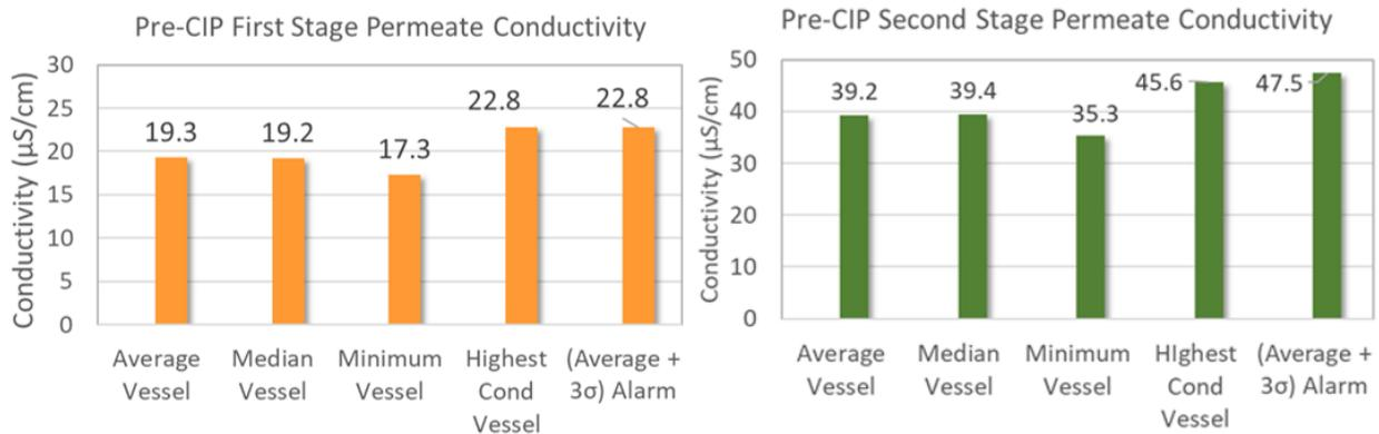
**Figure 6-10. Manual Conductivity Profile Prior to MS2 Dosing for Test 1 - Pre-CIP.**
