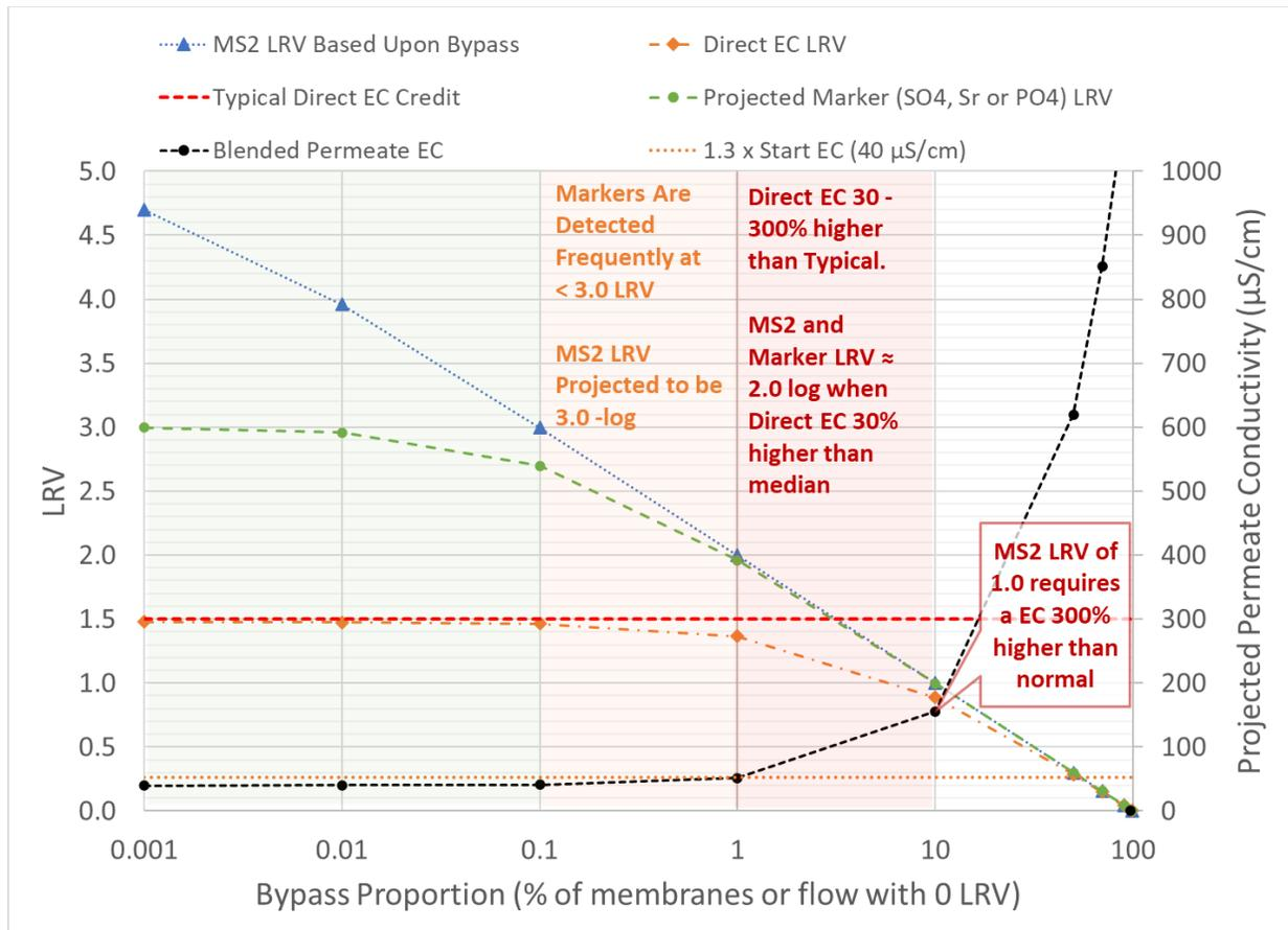
**Figure 9-1. Hypothetical Response of MS2, Marker and Conductivity LRV to Increasing Proportions of Bypass Flow.**
