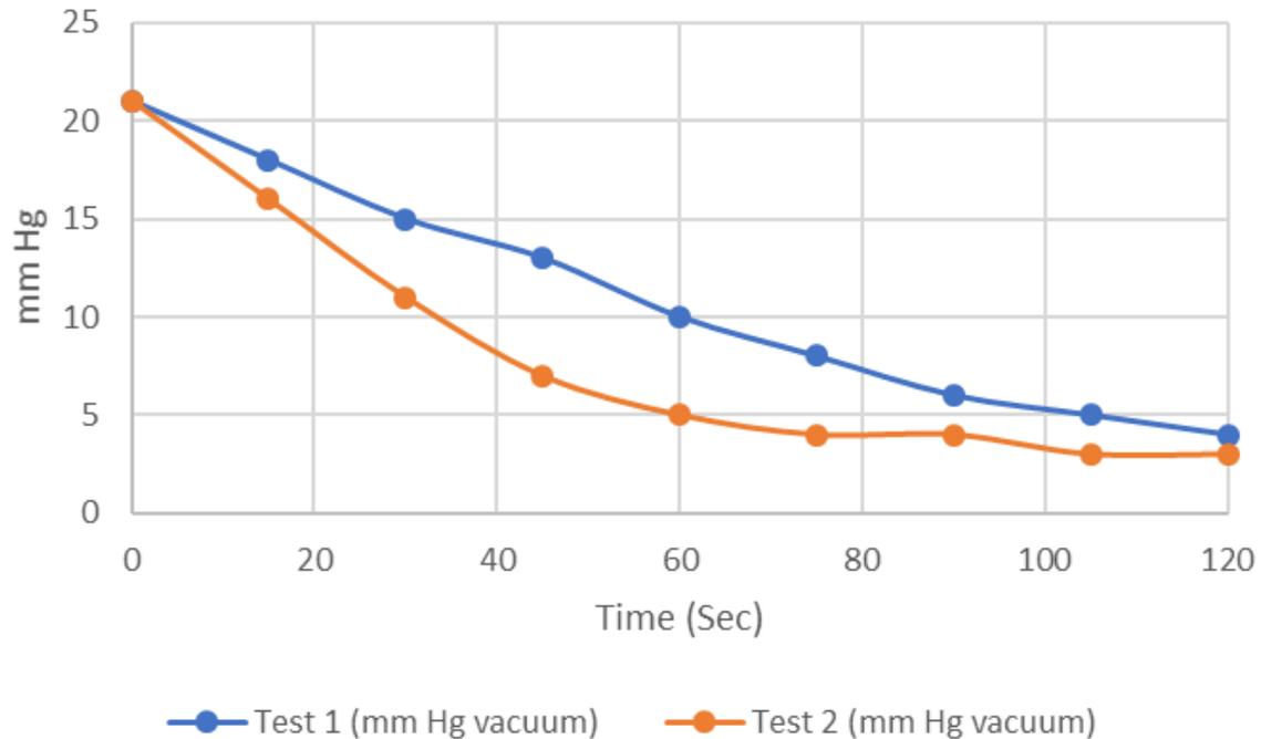
**Figure 4-12. Results of Vacuum Decay Test of Vessel 33.**
