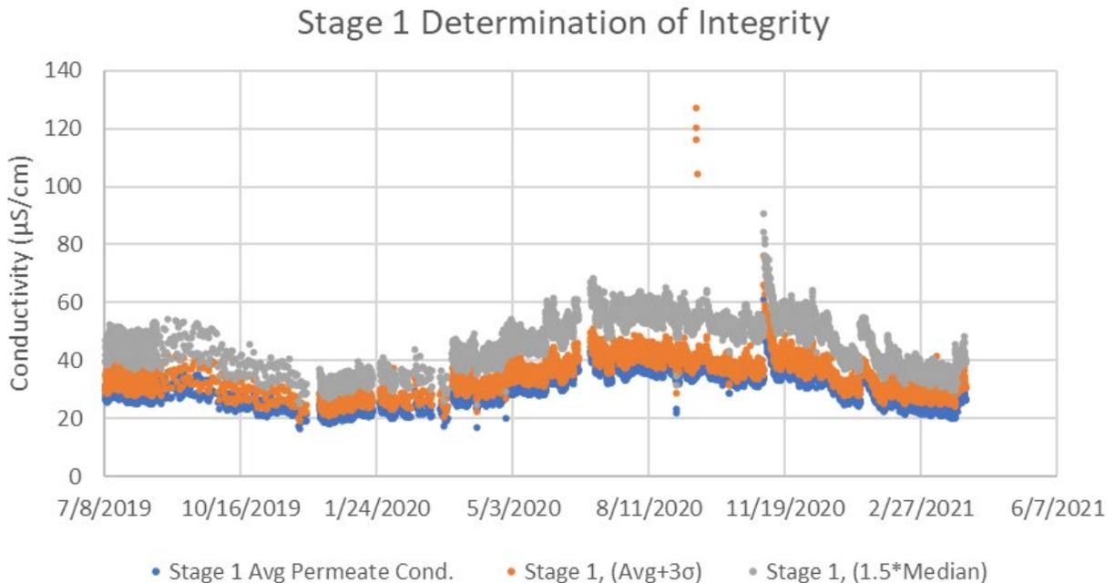
**Figure 4-14. YVWD Stage 1 Average Permeate Conductivity, Average +3 $\sigma$ , and 1.5\*Median.**
