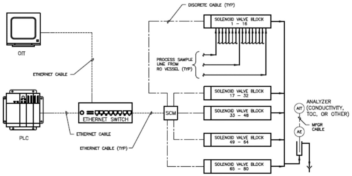
Figure 4-4. Schematic of Automated Conductivity Profiling Apparatus.
