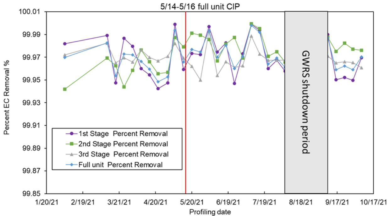
**Figure 5-6. OCWD Percent EC Removal Calculated Based on EC Profile Results for the 1st Stage, 2nd Stage, 3rd Stage, and Overall (Full Unit).**
