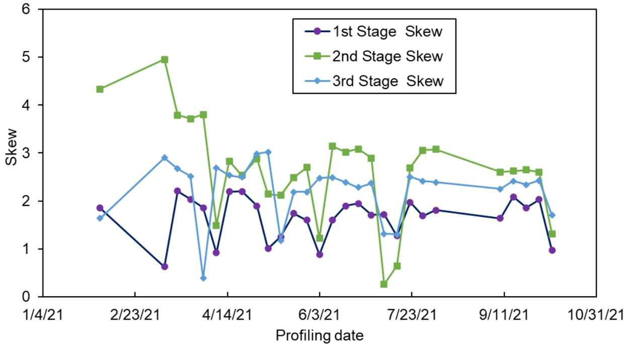
**Figure 5-2. The Stage Average Skew Calculated from the RO Permeate Conductivity Per Pressure Vessel for each Manual Conductivity Profiling Event (Approximately Monthly) at OCWD.**
