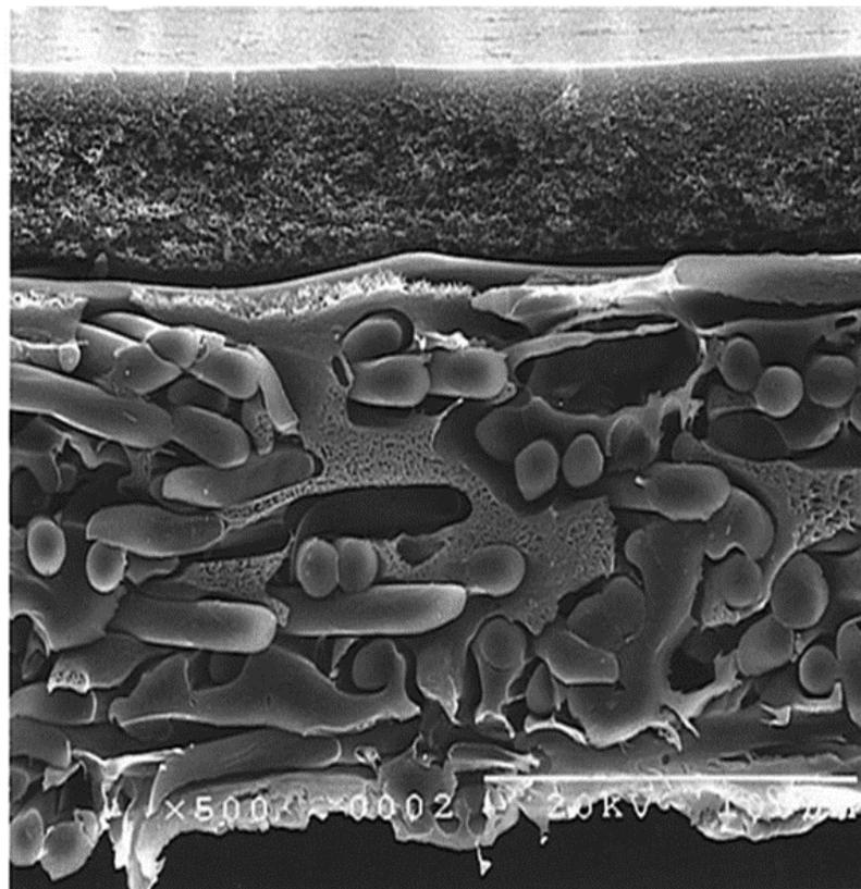
**Figure 1-2. Reverse Osmosis Membrane Cross Section.**
