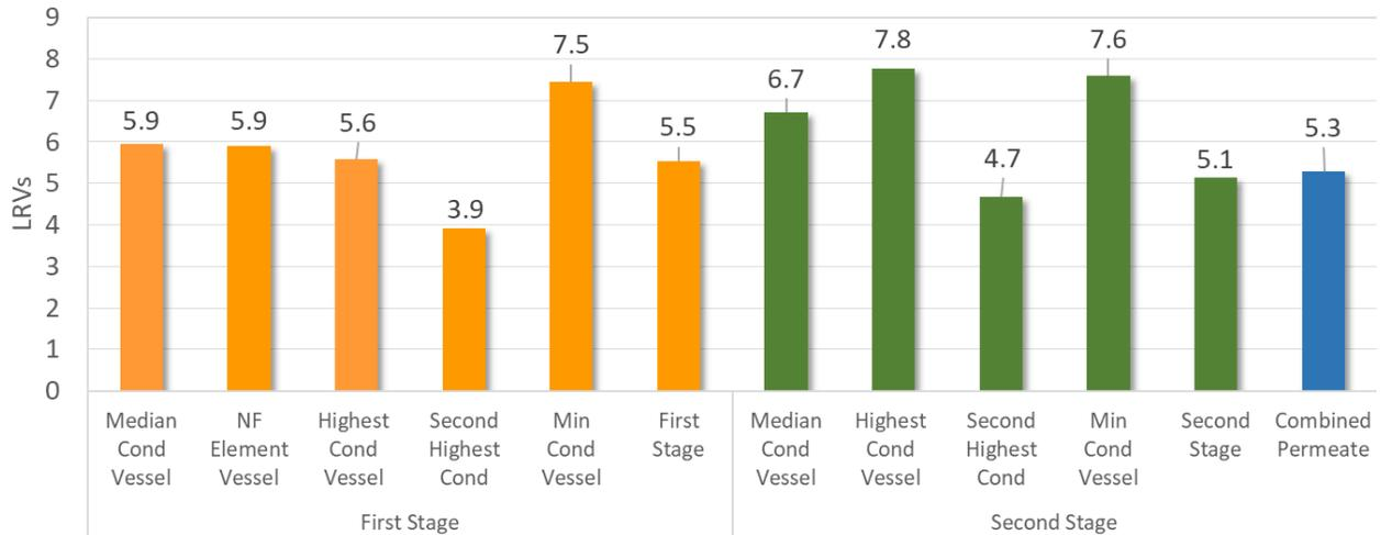
**Figure 6-17. MS2 LRVs Attained by RO System During Test 4 - NF Element Substitution.**
