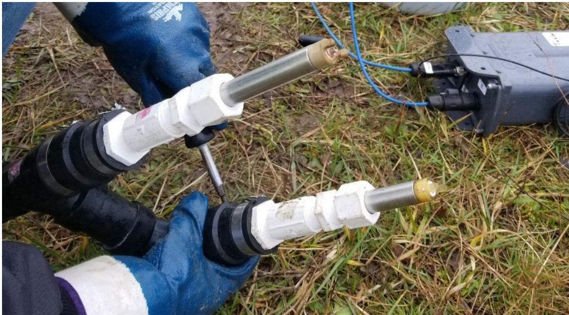
Figure A-9. Generic Sensor Holder with the Two Probes (pH and ORP).
