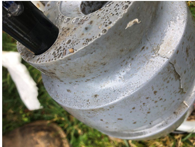
Figure 5-1. Corrosion and Damage to the Probe System.
