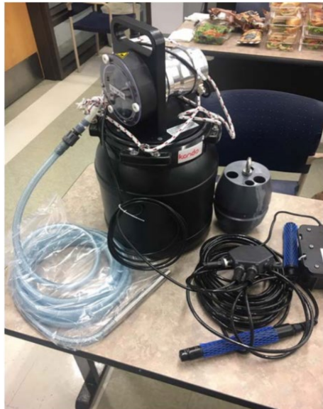
Figure 2-1. Kando Monitoring Equipment.
