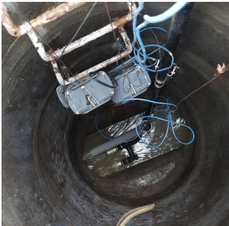
Figure A-8. Rag Guard Sensor Holder and Generic Sensor Holder Installed in the Same Manhole. This is showing the 'pronged' sensor holder initially used. The prong was eventually removed during the experiment to provide a gap between the sensor holders.
