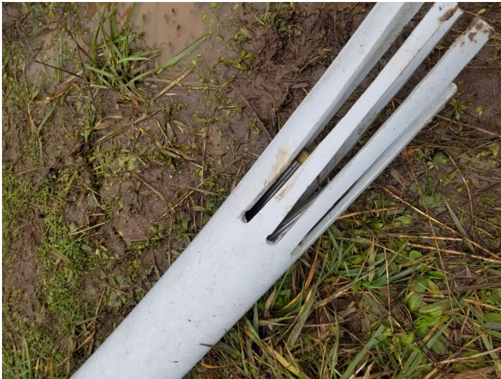
Figure A-7. Rag Guard Sensor Holder Showing the Probes as Installed in the Slats. Slats get wider with distance downstream.
