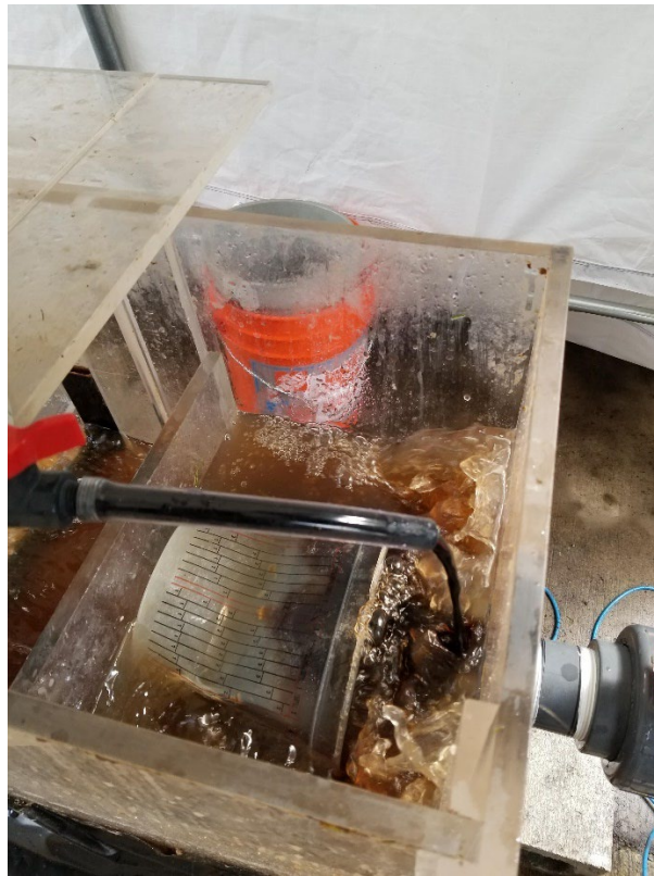
Figure A-3. Stilling Well on Front End of the Flume with Elevated Humic Acid Spiking Solution Dosing In Progress.
