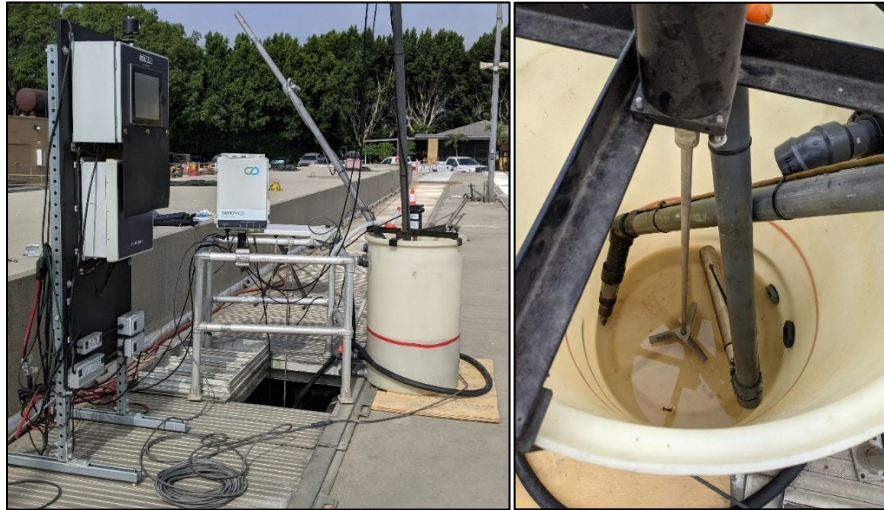
Figure 3-29. Challenge Testing Setup (left) and Plan View of Sensors in the Tank (right).
