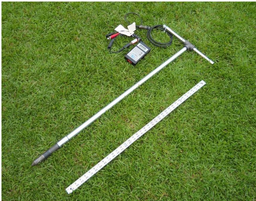
**Figure ES-1 Prototype Field LPR Probe from this project with annealed ductile iron rings**
