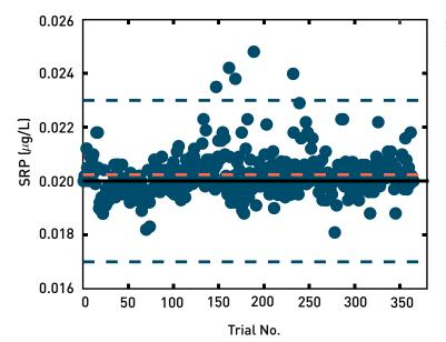
Samples prepared at 20  $\mu g$  P/L as orthophosphate sample. Samples measured during 2012.
