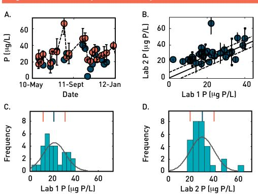
Figure 9-3 - Total Phosphorus (TP) Analysis of Pilot-Plant Membrane Permeates
