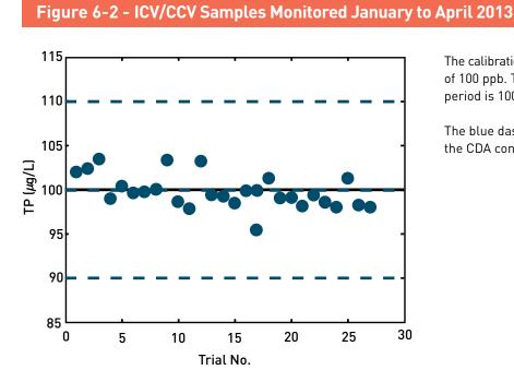
The calibration sample had a phosphorus concentration of 100 ppb. The mean of all 27 data points over this period is 100.
