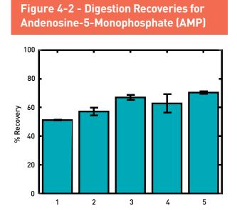
Digestion method indicated as the corresponding label number in Table 4-2.
