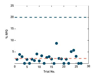
Effluent sample concentrations in the range 0.30 mg P/L to 1.1 mg P/L. Relative percent difference (RPD) calculated as in Equation 4. Data were monitored January to April 2013. Mean of the RPD data is shown as a red line.
