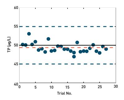
The LCS sample was prepared at 50 ppb phosphorus. The mean value is shown as a red dashed line and the blue dashed lines represent the control criteria limits (Table 6-1).
