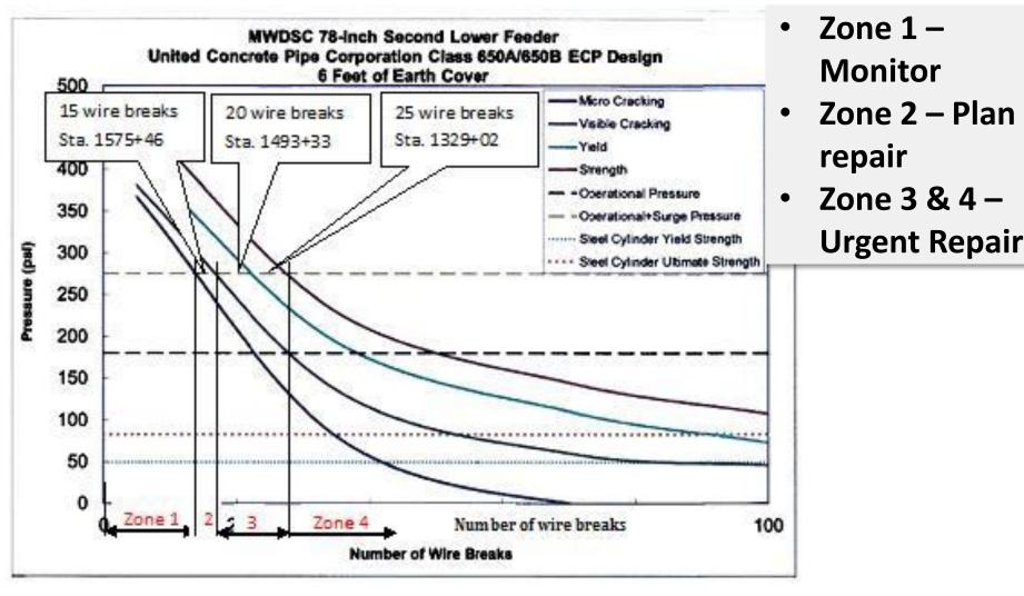
Figure ES.1: Performance Curve for the 78-Inch Class 650A/650B Pipe Design
