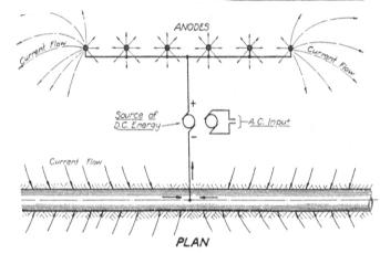
Figure 1. General Arrangement Of Cathodic Station.
