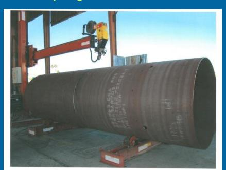
The double-v-groove complete penetration circumferential butt joint can be radiographically tested.
