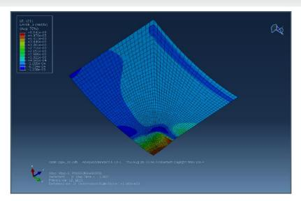
Figure 3 – Strains in the fiber direction of the inner layer of CFRP at 500 psi pressure. Note maximum strain of 0.55 percent.
