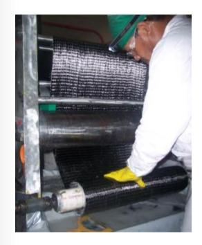
Impregnate Carbon Fiber fabric with Epoxy
