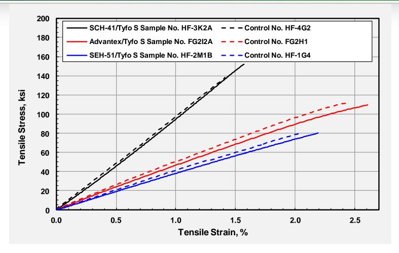
Typical stress-strain curves for Tyfo Fibrwrap composite control samples and 15-yr Yolo Causeway exposure samples.
