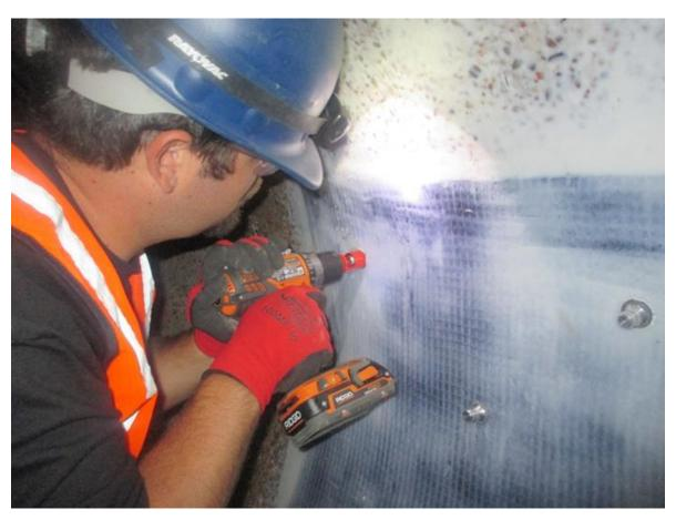
Drilling the holes to set the test pucks for adhesion tests
