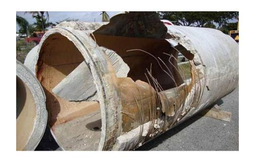
**Ruptured 54-inch PCCP water transmission main**
