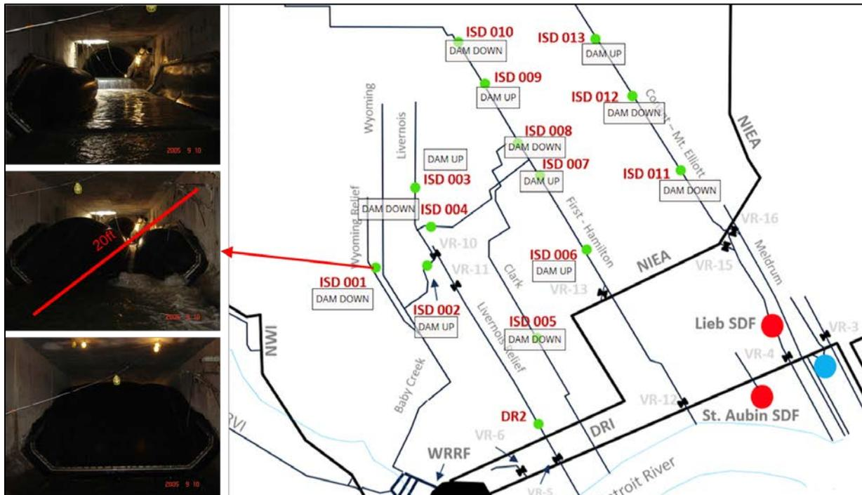
Figure 1. Detroit sewer network is equipped with inflatable in-line storage dams (green circles) that can use storage capacity in the pipes to regulate wet-weather flows.
