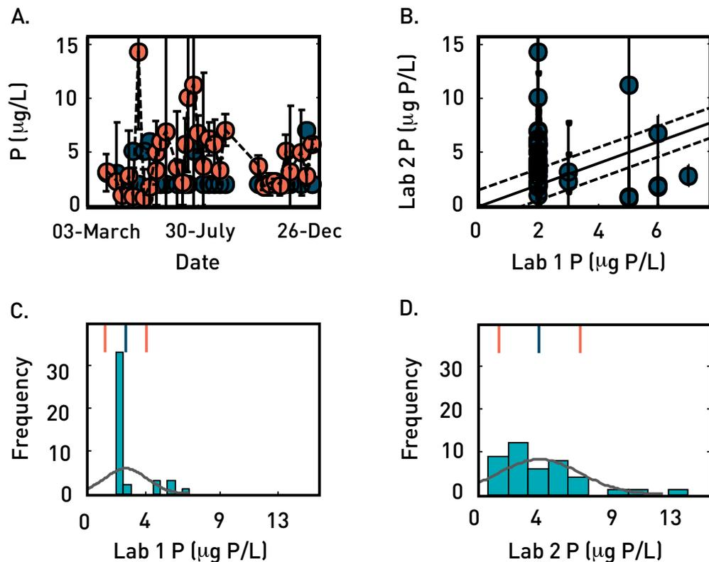
Samples measured by two different analytical laboratories. Laboratory 2 did three replicate measures on each sample and corresponding 95% confidence intervals are shown.
