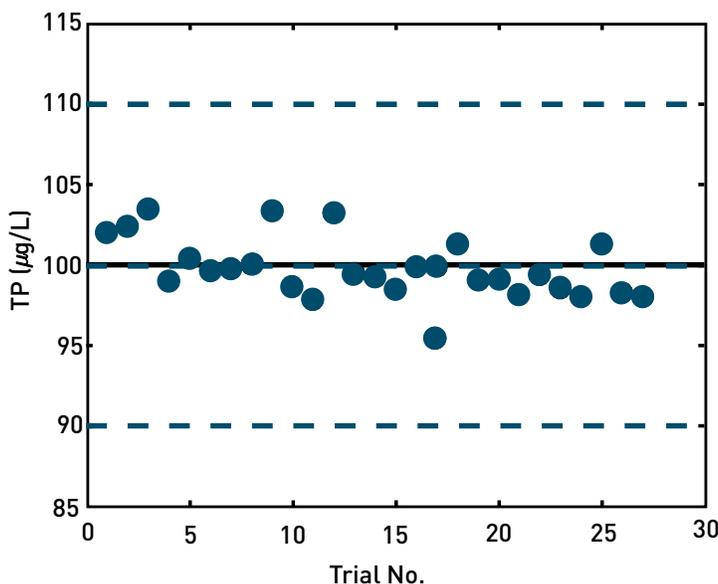
The calibration sample had a phosphorus concentration of 100 ppb. The mean of all 27 data points over this period is 100.
