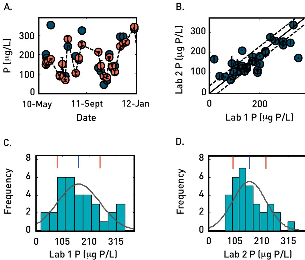
Samples measured by two analytical labs. Laboratory 2 did three replicate measures on each sample and corresponding 95% confidence intervals are shown.
