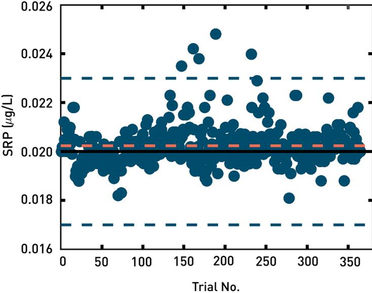
Samples prepared at 20 µg P/L as orthophosphate sample. Samples measured during 2012.
