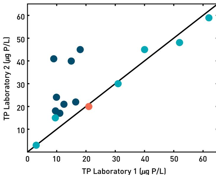
Laboratory 2 corresponds to Wilfrid Laurier University and measurements are shown as blue circles using the initial ascorbic acid method, red circles using ICP-OES, or aqua circles using the improved ascorbic acid method.
