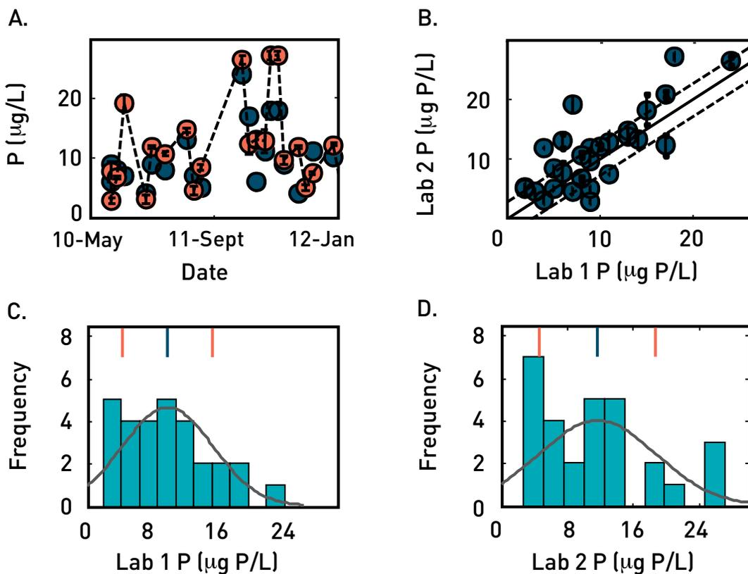
Samples measured by two analytical laboratories. Laboratory 2 did three replicate measures on each sample and corresponding 95% confidence intervals are shown.
