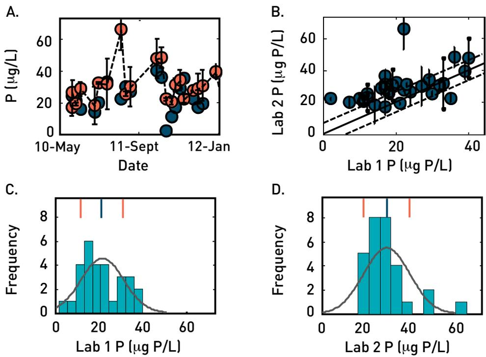
Samples measured by two different analytical laboratories. Laboratory 2 did three replicate measures on each sample and corresponding 95% confidence intervals are shown.
