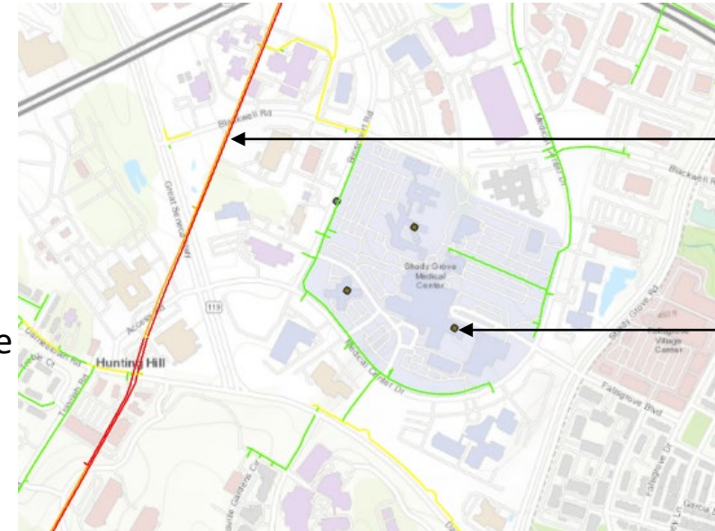
High consequence pipe near critical facilities (hospitals)
