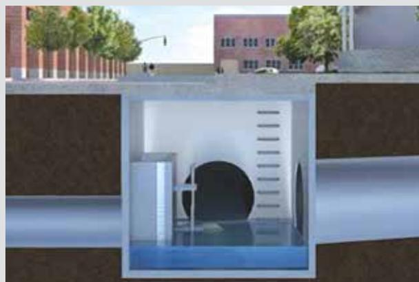
*Cities: High-Performance Green Infrastructure* (INFR1R11), showed that technologies significantly lowered contributions to CSOs, reduced stormwater runoff, and retained stormwater for onsite use—helping to push the technology into full commercialization the same year.
