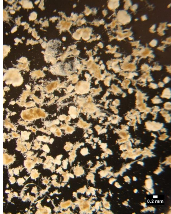
Densified sludge: SVI ~50 to 90 May contain some granules >200 \mu\text{m}
