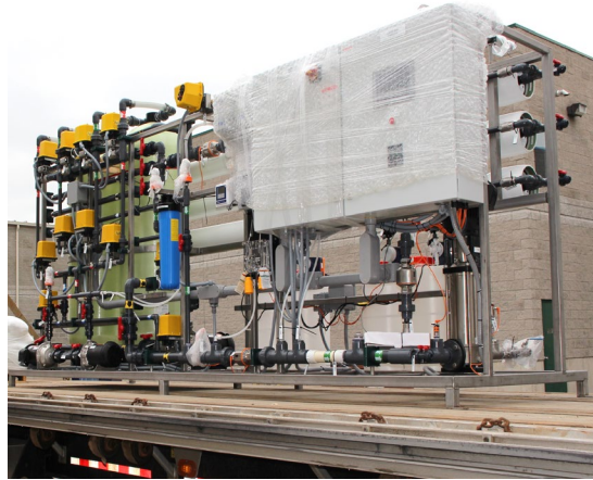
Reverse Osmosis Plant: Canadian food & beverage manufacturer
