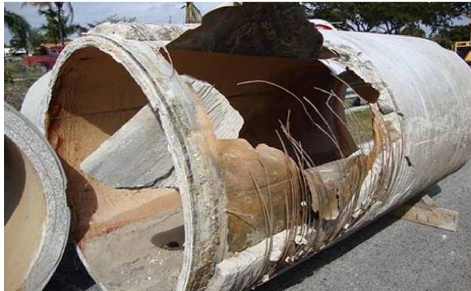
**Ruptured 54-inch PCCP water transmission main**
