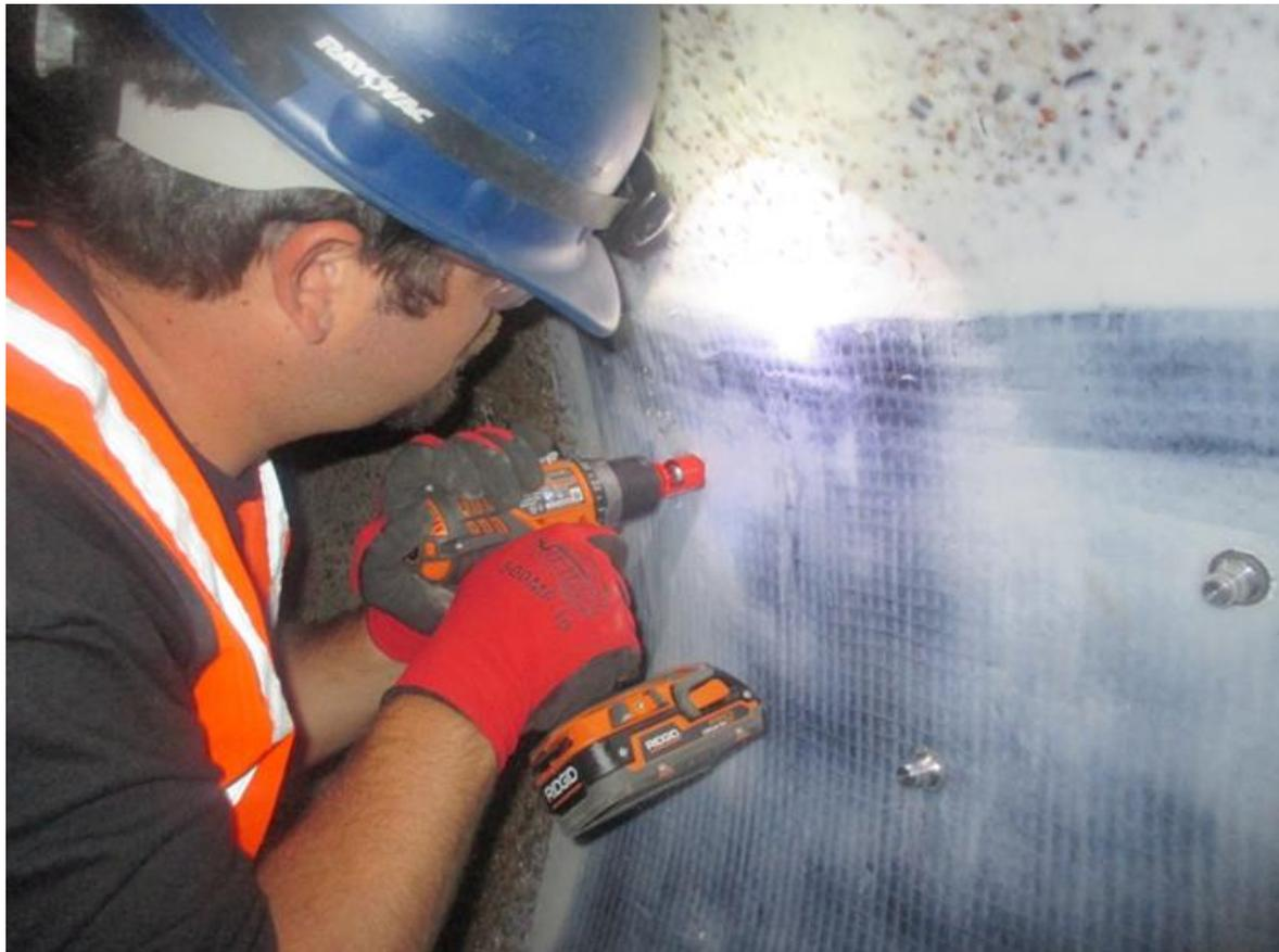
**Drilling the holes to set the test pucks for adhesion tests**
