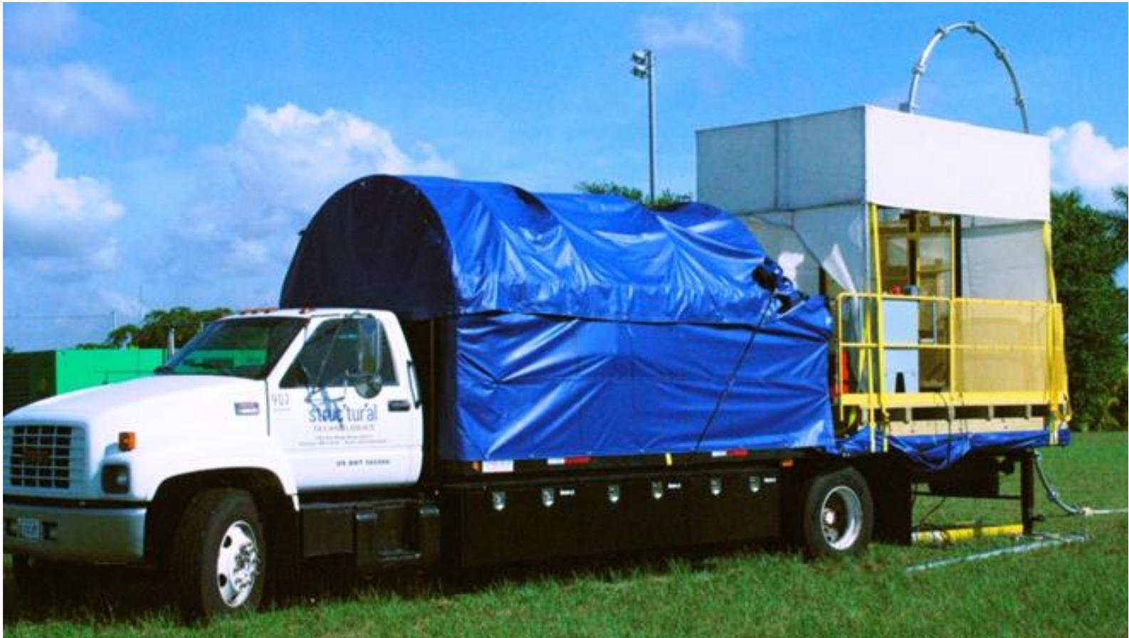
**Truck mounted unit for Hybrid FRP System**
