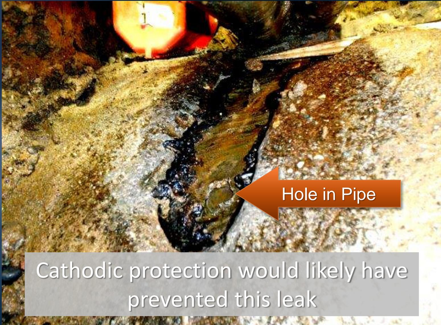
Cathodic protection would likely have prevented this leak
