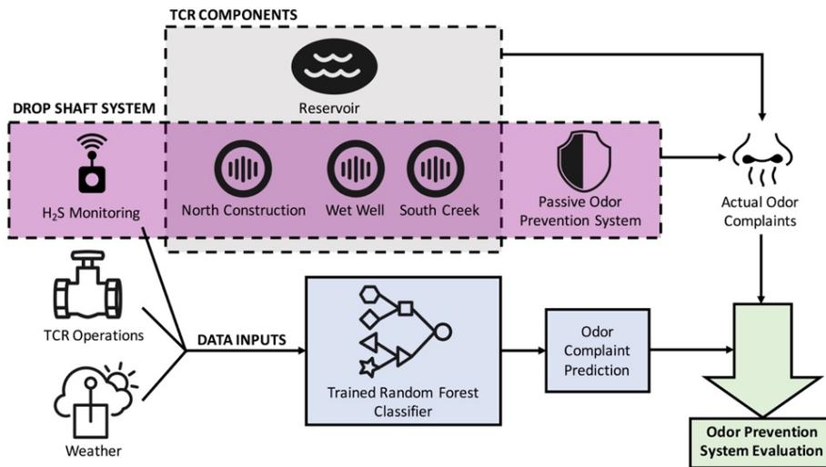
**Figure 4. Algorithm deployment within the updated odor control system at TCR drop shafts**
