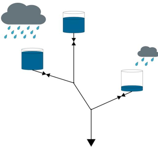
Figure 3. A market is comprised of upstream buyers and a downstream seller. Buyers have storage volume and a control element, allowing them to regulate their outflow. At each timestep, discharge from each buyer is determined within the market.
