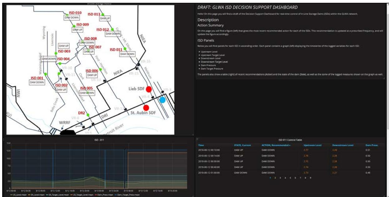
Figure 5. GLWA in-line storage dam dashboard provides real-time recommendation of control actions.
