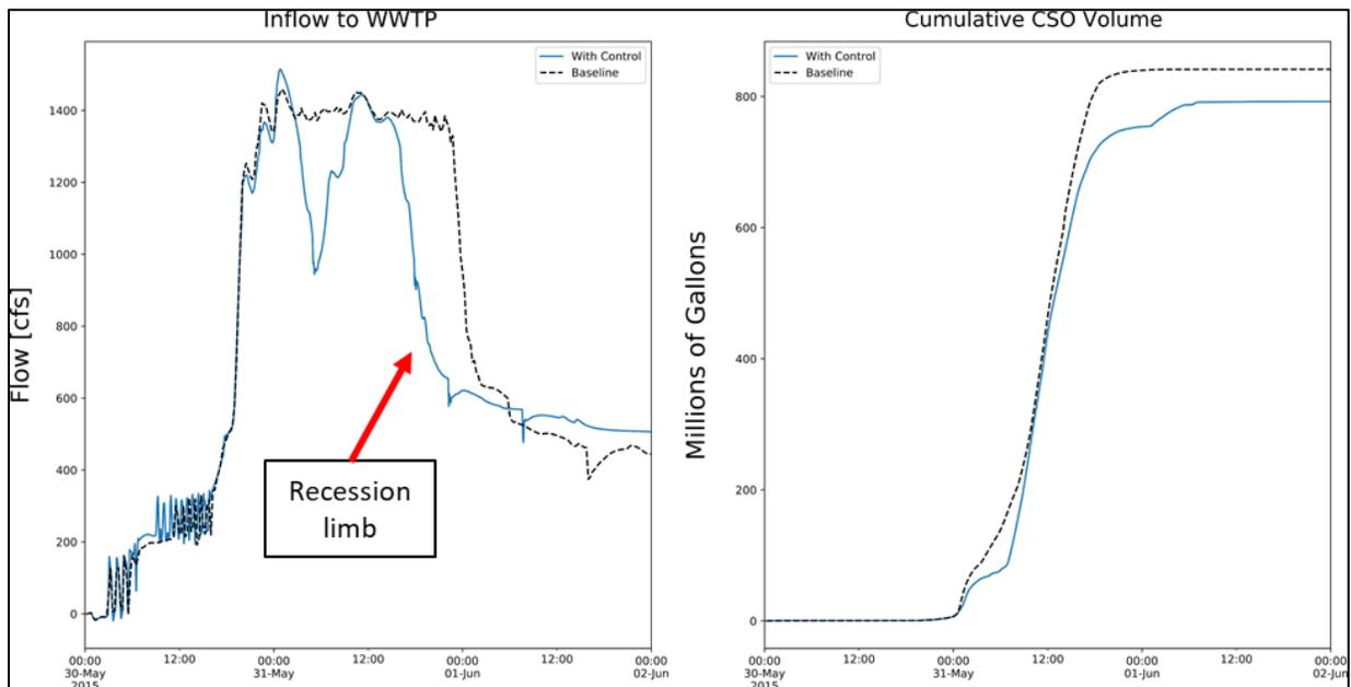
Figure 4. Timeseries results for the May 30, 2015 storm event. Dynamic control resulted in a reduction of ~100 Million Gallons of combined sewer overflow as compared to baseline.
