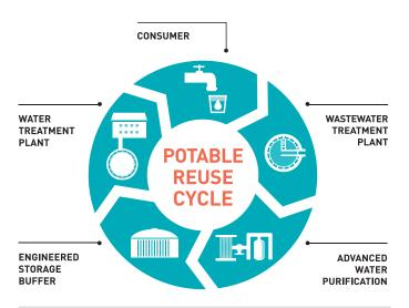
Potable reuse is the process of taking treated effluent from a typical wastewater treatment plant and purifying it further with advanced technologies.
