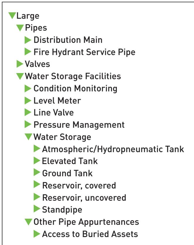
Figure 1. Simplified tiering of distribution system assets
